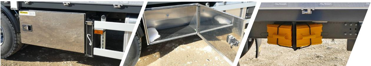
A large stainless steel box is installed on the left and right side. Stabilizer plate holders and wheel chocks are mounted ready to hand.
