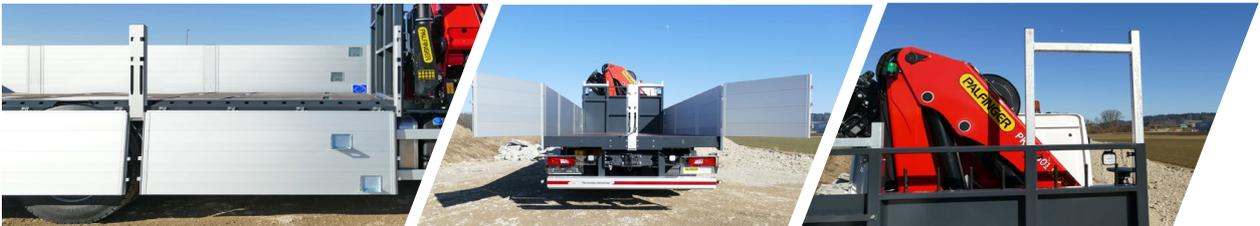
The platform is framed by side walls made of anodized aluminium side walls. At the rear there are 2 side-hinged doors, which can be opened and dismantled individually. The front wall consists of a solid steel frame with 2 galvanized extensions for the transportation of long goods.
