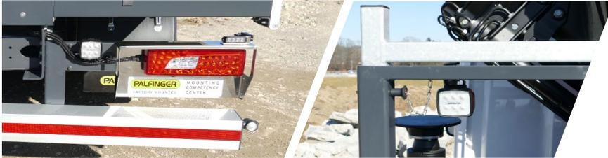
2 LED working lights and 6 LED reversing lights provide optimal illumination of the site. In addition, this vehicle is also equipped with 6 flashing lights and 2 outline lamps.
