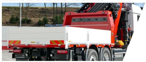
The platform with integrated cutouts for the mudguards is attached laterally to the subframe to keep the loading height as low as possible. The PALFINGER design front wall is not only convenient but also a real eye-catcher.
