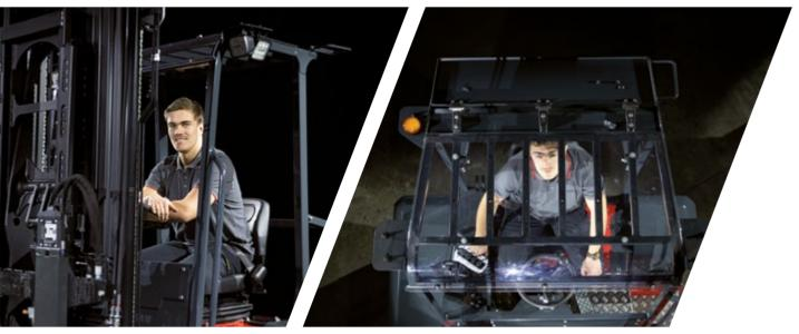
Centrally positioned seat with large-scaled and visibility roof  Driver protection frame fulfills ROPS/FOPS criteria
