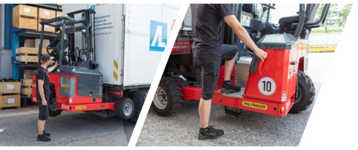
• Ideally placed ground controls at the rear for fast and safe mounting and dismounting at ground level.
