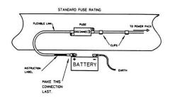
Protect the fuse from road spray to stop terminal corrosion.
