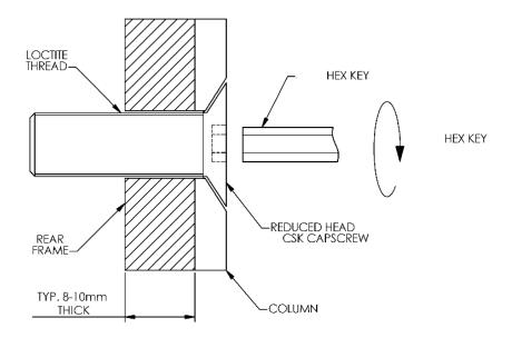
Ensure threads are clean before using Loctite.
