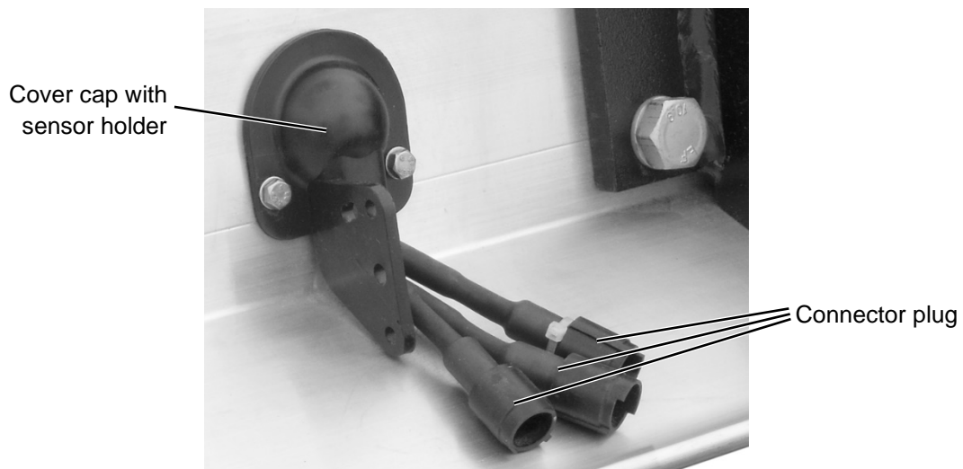
Figure 40: Cover cap with sensor holder for tilt sensor B15
