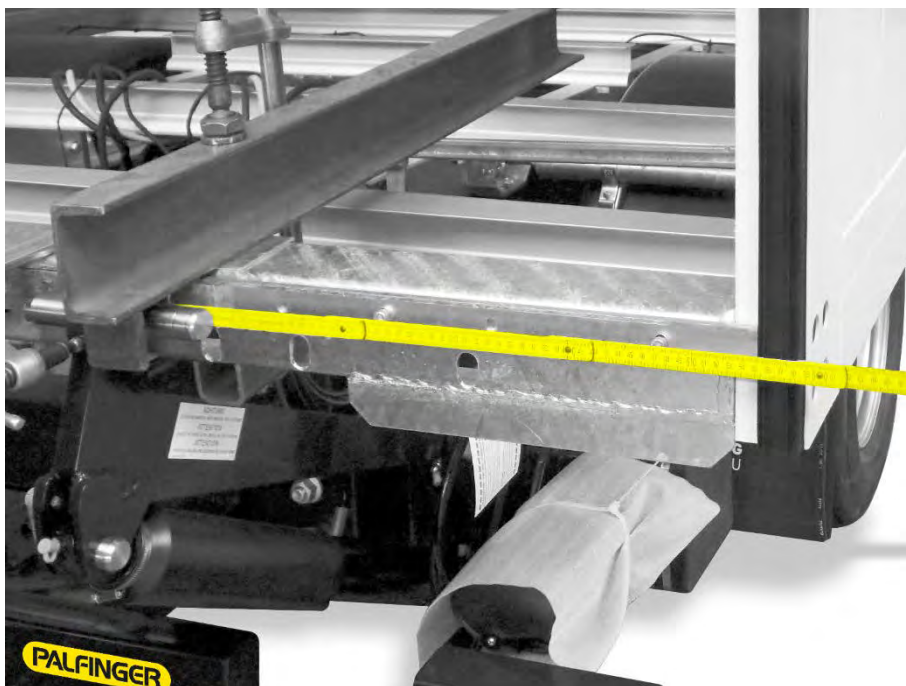
Figure 18: Check the central position of the lifting mechanism (2)
