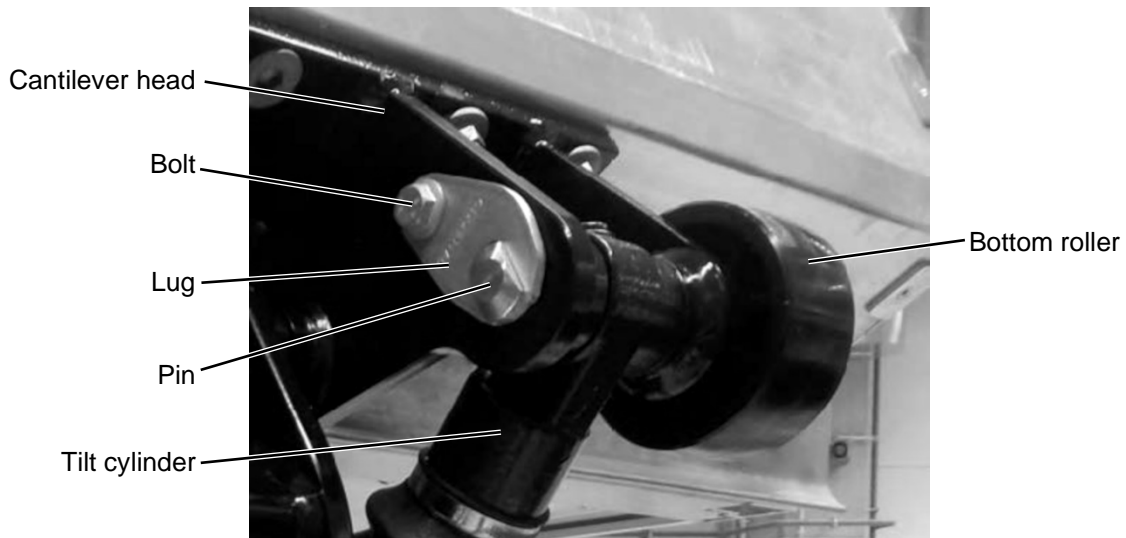
Figure 37: Bolting the tilt cylinder
