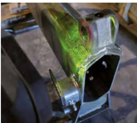
The components are inspected for structural damage by means of an MT test (magnetic particle test).
