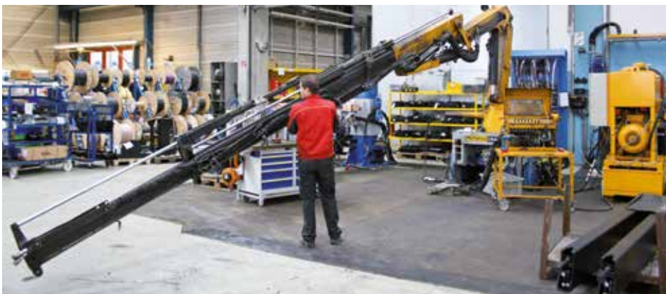
The attachments are removed. The main components are disassembled and labelled.
