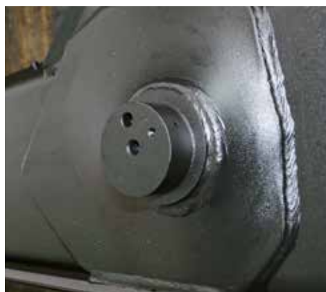
The components are given a CDP (cathodic dip paint) coating. Cathodic dip painting provides outstanding mechanical and chemical protection, which also extends into the cavities of the components.
