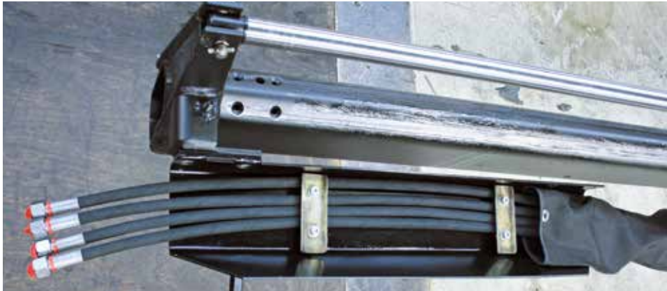
Attachments are refitted. All wear parts, such as hydraulic hoses, are newly manufactured.
