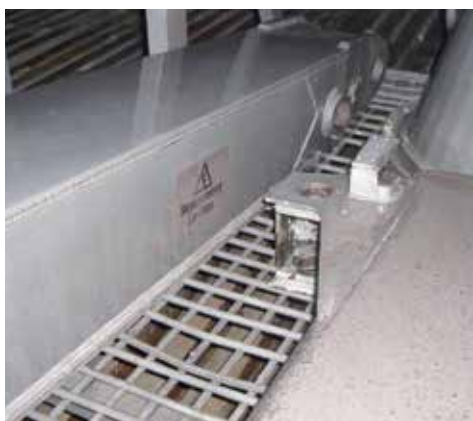
The components are stripped of paint, cleaned and conserved using a chemical dipping method.
