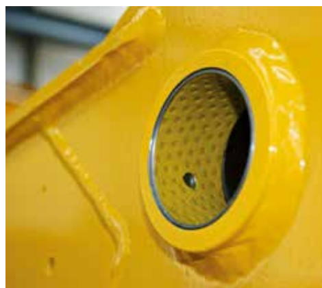
All moving parts are given new bearings.
