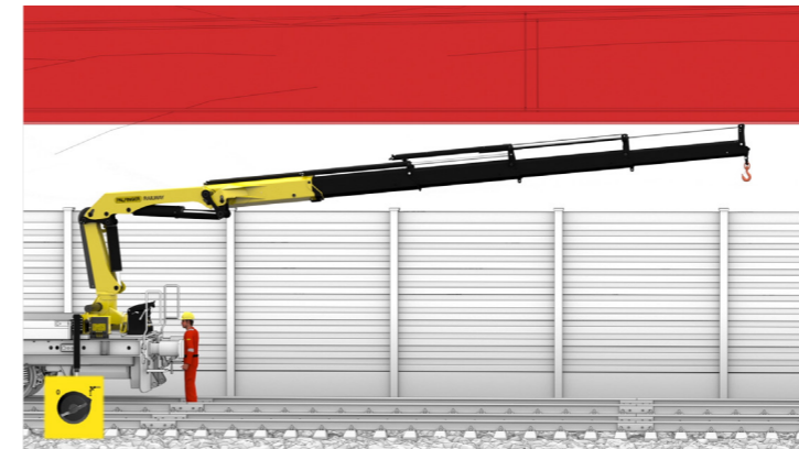
Height Limiter pld-compliant acc. to EN 13849
