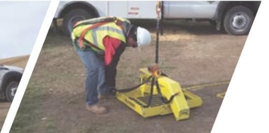
4 REMOVE THE LOAD HARNESS FROM THE PLATFORM
