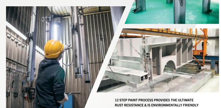
Components are cleaned and pretreated with a phosphate conversion coating to prepare the product for electrocoating. When dipped into a paint bath, direct current is applied between the product and a counter
