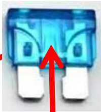
Replace with 15A ATC fuse (BLUE) if metal bridge is broken.
