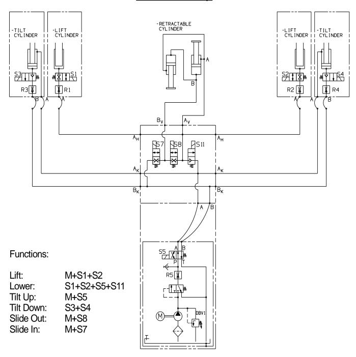
S1, S2 on lift cylinder and S7, S8 on push pull valve block are double acting release valves: They have to be activated for fluid to go through them in either direction
