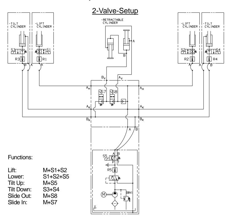
S1, S2 on lift cylinder are double acting release valves: They have to be activated for fluid to go through them in either direction
