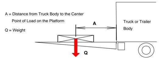
Figure 2: Center Point of Load
