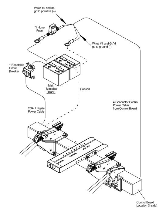
$<sup>^*\</sup>mbox{In-Line}$  ATC Fuse: 20 Amp. Replace with same amperage fuse when necessary.
