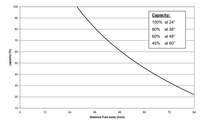
Figure 3: Load Diagram (ILU 40, 50)
