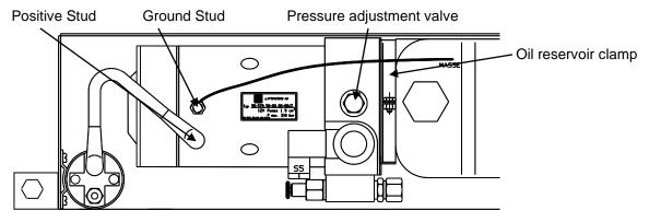
Figure 7: Power Pack (Top View)
