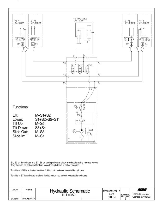
Figure 11: Hydraulic Schematic
