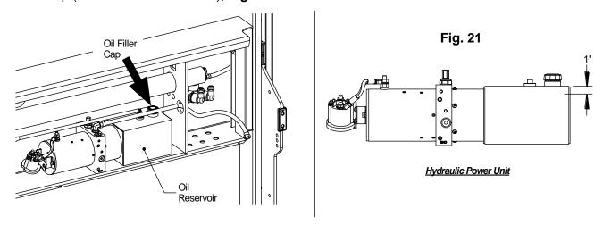
All ILM liftgates come with Hydrex MV Arctic 15 hydraulic fluid.
