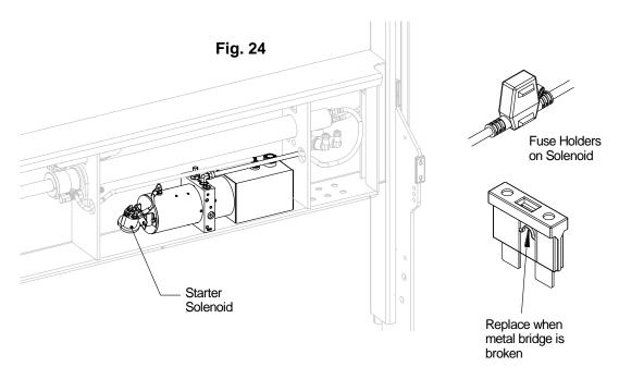
In-Line ATC Fuse 15 Amp at solenoid. Replace with same amperage fuse when necessary.
