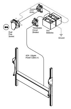
Battery Wiring - Dual Pole - Trailer
