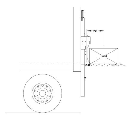
By increasing this distance "A" the maximum load of the lift gate is decreasing. Make sure not to overload the liftgate. Place the cargo in the middle of the platform. Operating a gate with a misplaced load may cause serious damages or even injuries to the operator.
