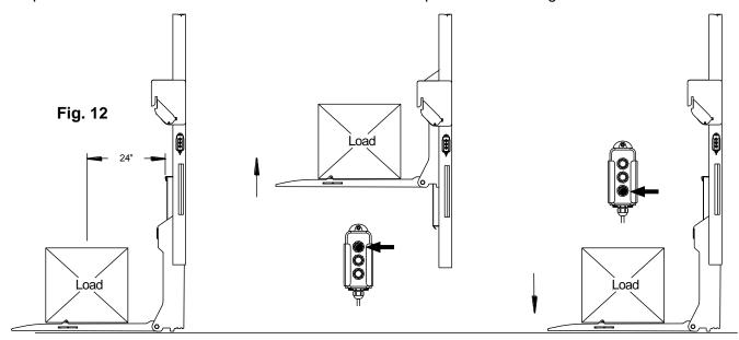
5. To store the platform, Press the **Up** button to raise the platform approximately 12" from the ground. Press and hold the **Shift** and **Up** buttons simultaneously until the platform is parallel to the columns, **Fig. 13**. Press the **Up** button to raise the platform until the platform locking ears are positioned in the locking plate and the storage safety lock is engaged.
