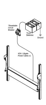
**Battery Wiring - Truck**
