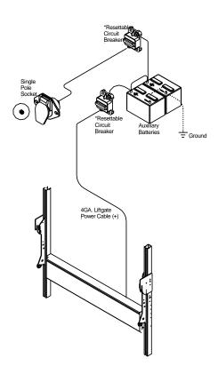
Battery Wiring - Single Pole - Trailer
