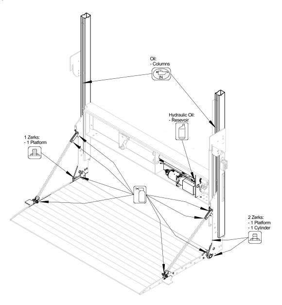
Grease fitting, 2 for deck, 2 for power closing.
