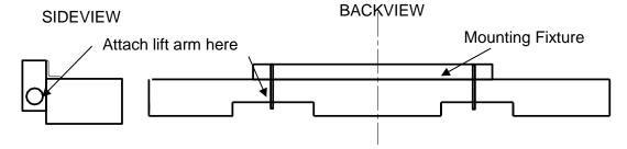
Figure 5.1: Mount fixture welded to rear sill
