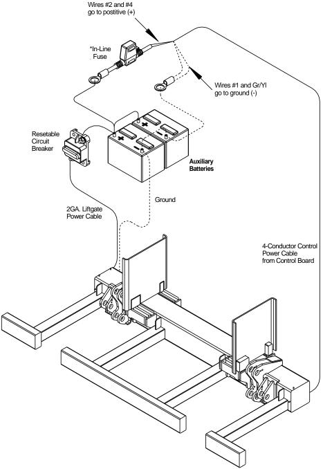
\*In-Line ATC Fuse: 20 Amp. Replace with same amperage fuse when necessary.
