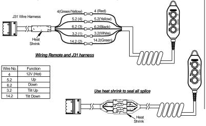
3. Test each function to verify the control is functioning as intended. Use the provided wire clamp to secure the control harness from any tugging. Apply the decal within the vicinity of the control. Installation complete.
