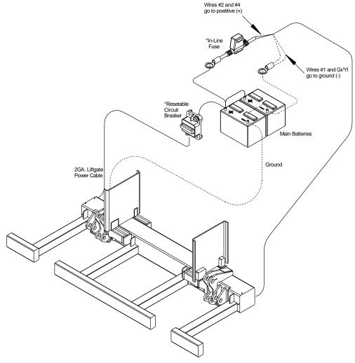
\*In-Line ATC Fuse: 20 Amp. Replace with same amperage fuse when necessary.
