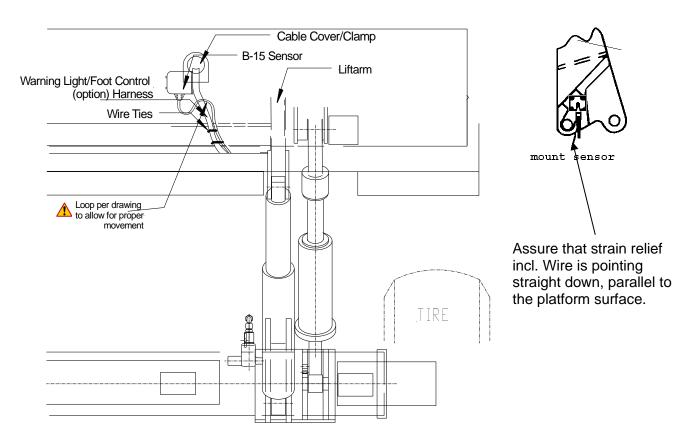
Figure 5.4: B-15 Sensor and warning light cable installation and placement
