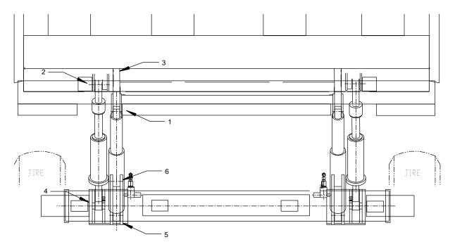
Figure 7.1: Lubrication Points (opposite direction on curb side )
