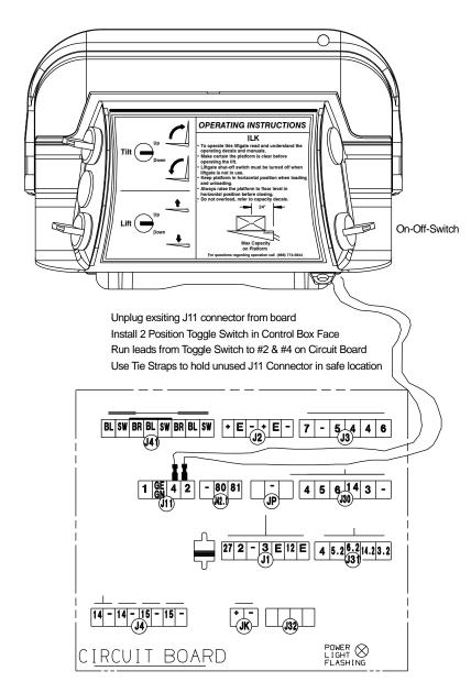
The Circuit Board is located behind the rubber cover on the curb side of the 7" x 7" mount tube.
