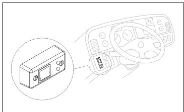
Place cab shut off in view of the driver and within reach from the ground.
