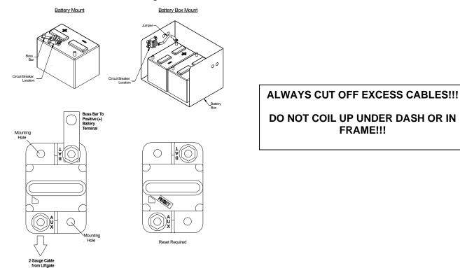
Figure 6.1: Circuit Breaker installation
