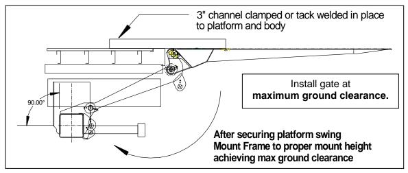
Figure 5.3: Platform install without fixture
