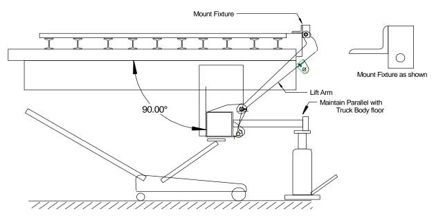
Figure 5.2: Mount frame alignment with fixture
