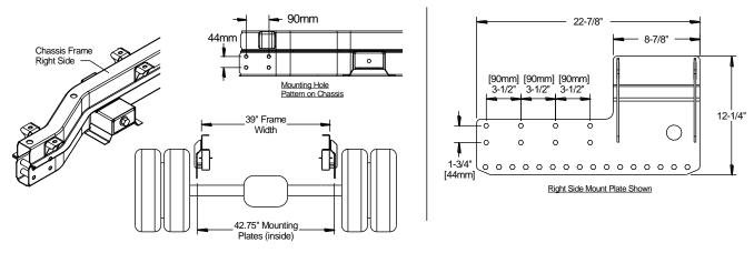
2. Mount Plates: Mount the mount plates to the chassis using the hole pattern of the chassis frame. Add four spacers between the chassis frame and mount plates. Secure the mount plates using M12x90mm hex head bolts. Do not tighten bolts completely. Attention: The body on a 170" wheelbase could extend further back than on a 144" wheelbase. An alternative to mounting the liftgate on a 170" wheelbase is to use the left side mount plate on the
