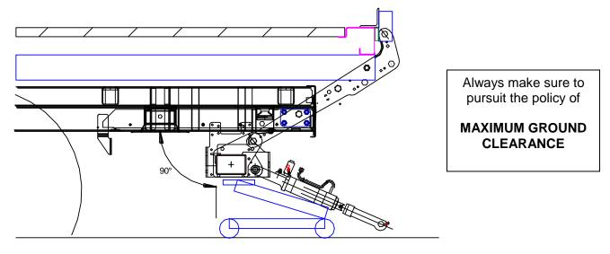
Mount frame alignment with fixture
