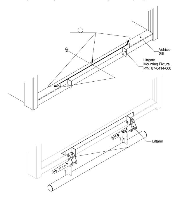
Mount fixture welded to rear sill
