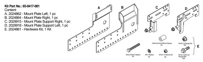
1. Chassis: The hole pattern at the end of the chassis frame measures 90mm x 44mm. The mount plates have three mounting options with the same dimensions of 90mm x 44mm.
