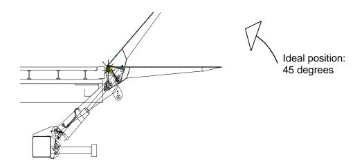
Attaching of platform with tilt cylinders
