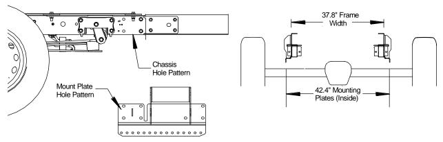
2. Mount Plates: Install the mount plates on the chassis using the hole pattern of the vehicle chassis frame. Drill three ø20mm holds to install the three spacers between the chassis frame and mount plates. Secure the mount plates using M12x90mm hex head bolts. Do not tighten bolts completely.
