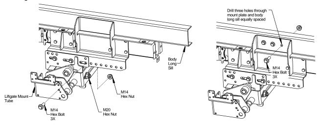
Make any adjustments to the mount tube using the hole pattern on the mount plate. The mount plates allows for up to 10.5" of adjustments. After any adjustments, torque all bolts to their corresponding values shown.
