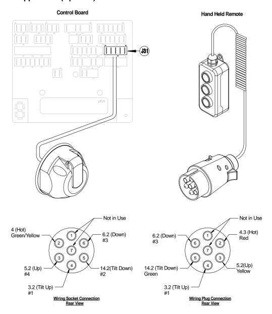
Hella Plug & Socket wiring for Hand Control
