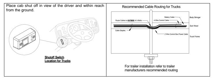
2. Lead the <u>4-wire cab switch</u> together with the battery cable and the 4 wires for the control power to the batteries along the sub-wood. Secure the cable every 12 inches against the sub-wood with cable staples. Run only the <u>cab switch</u> into the cab. Battery cable and 4 wire control power cable will go directly to the truck battery. (#2 and #4 go to positive post **with an inline 20 amp fuse**; #1 and green/yellow go to negative post).
