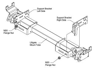
4. After installing the support brackets secure the support brackets to the mount plates using the M14x1.5x45mm flange bolts as shown, do not tighten bolts completely. Tie the mount plates to the body long sill by drilling three additional holes through the mount plates and body long sill. Use M14 flange bolts and nuts.
