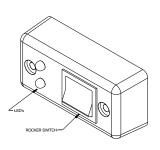
In Cab ON/OFF Switch (Truck)
