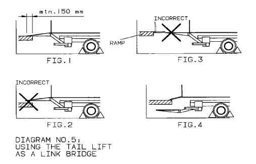
$\rightarrow$  Move platform under the ramp and apply a cantilever drive-over dock plate (Fig. 4).
