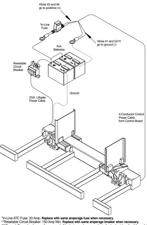
\*\*Resetable Circuit Breaker: 150 Amp Min. Replace with same amperage breaker when necessary. \*\*\*Ground: For optimal grounding, ground all batteries and power units to the body side rails of the vehicle. NOTICE: DO NOT attempt to jump in-line fuses with other objects other than the specified fuse. Do not increase the amperage rating of fuse. Serious harm to the liftgate will result when standard practices are not followed.
