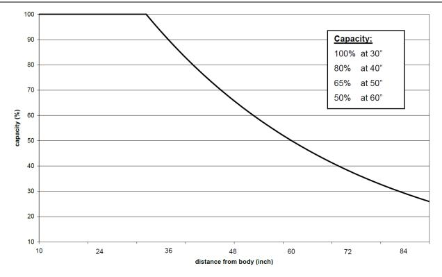
Figure 4: Load Diagram (ILK Plus 44 to 66)
