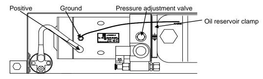
Figure 6: Power Pack (Side and Top View)
