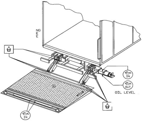
The gate has 12 grease zerks. On each side are 6 zerks. 3 in the mount frame area and 3 in the cylinder/platform area.
