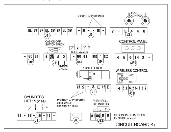
Figure 2 Plug setup on PC - Board
