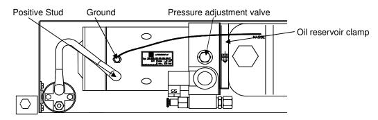
Figure 7: Power Pack (Top View)
