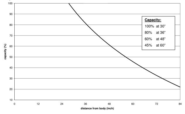
Figure 3: Load Diagram (ILFP 30 and 40)
