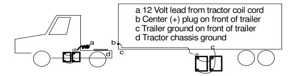
Testing of full system using a battery load tester:
