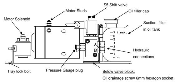
Figure 6: Power Pack (Side View)
