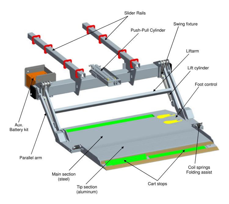
Figure 1: ILFP Slide lift
