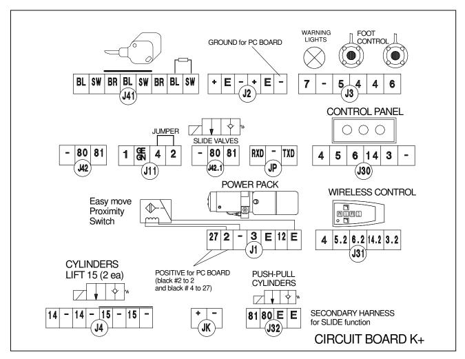
Figure 4 Plug setup on PC - Board
