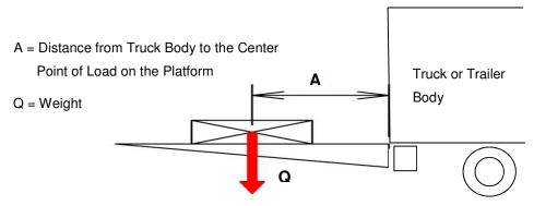
Figure 2: Center Point of Load
