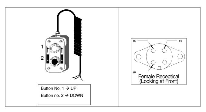
Figure 4: Hand Held Remote Control with Plug & Socket Wiring
