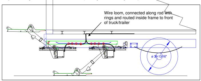
Figure 12 Power cable routing on passenger side
