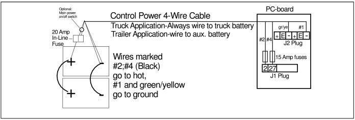
Figure 13 Board control power wiring connection
