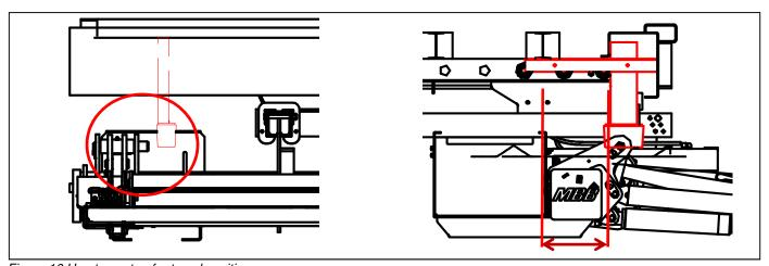
Figure 16 Up-stop setup for travel position
