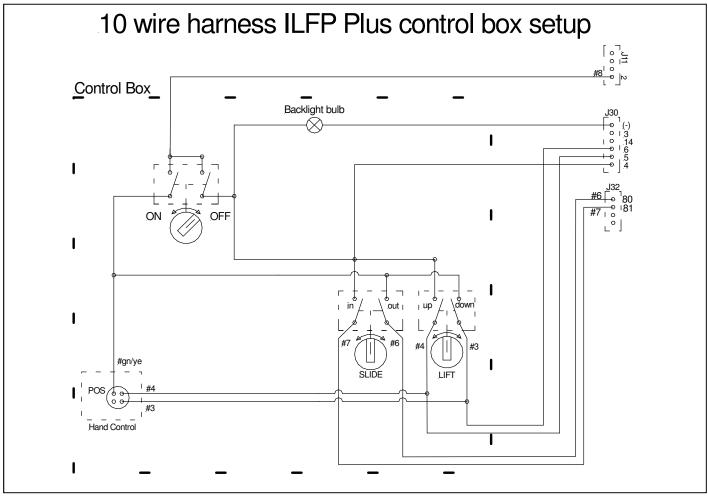
Figure 30 Control box wiring schematic
