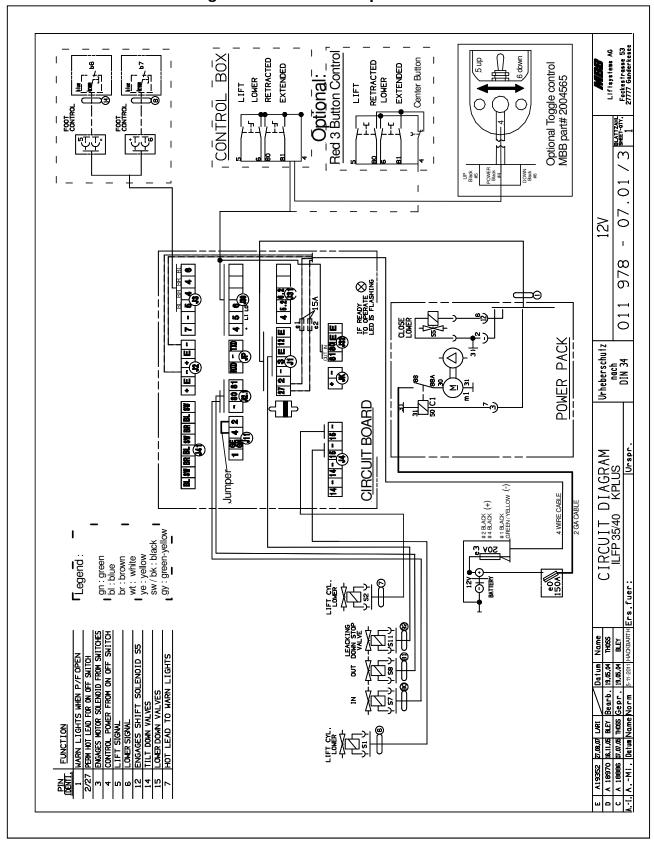
Figure 26 Control board wiring schematic
