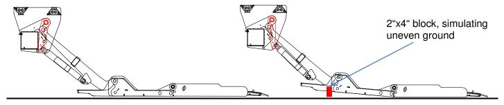
While swing arm is detaching from main frame lift cylinders keep retracting to compensate for rotation of platform. Platform stops lowering down when main section meets ground or cylinders are completely retracted.
