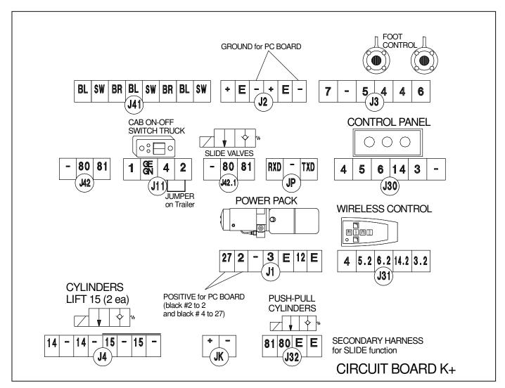
Figure 27 Plug setup on PC - Board
