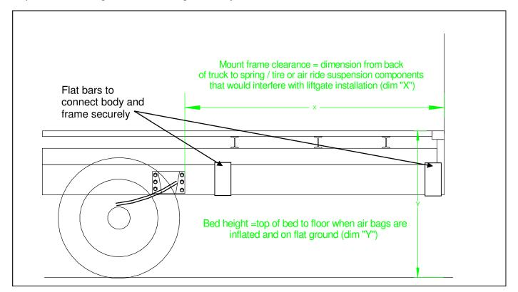
Figure 4 Mounting clearance
