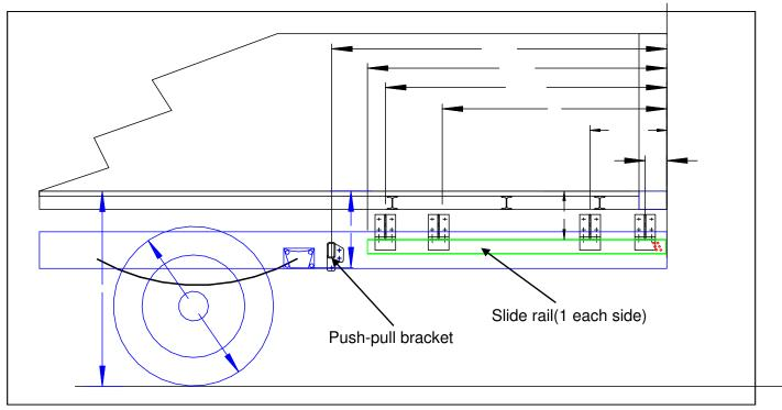
Figure 7 Slide rail and push-pull installation
