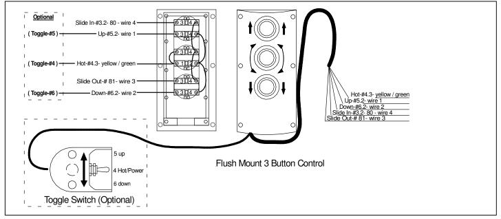
Figure 18 Flush mount Control box wiring
