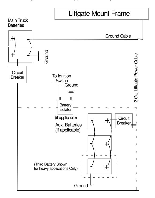
Figure 20 Main wiring - truck setup
