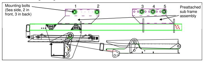
Figure 10 Rapid mount bolt-on setup
