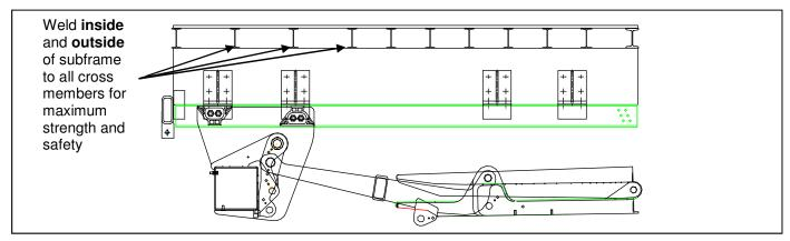
Figure 11 Quick mount weld-on setup
