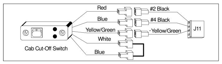
Figure 24 Cab Cut-off switch connection
