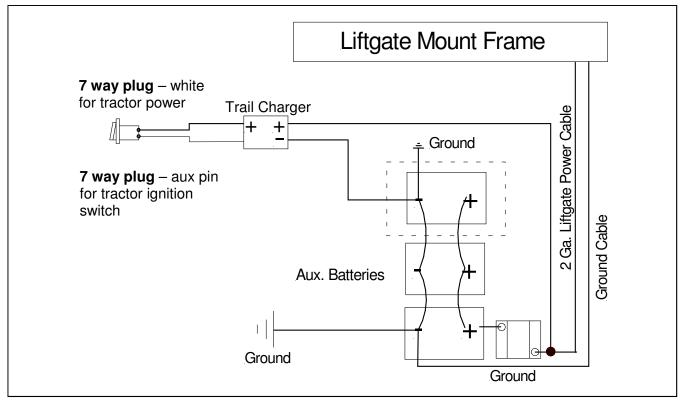
Figure 23 Trail charger wiring
