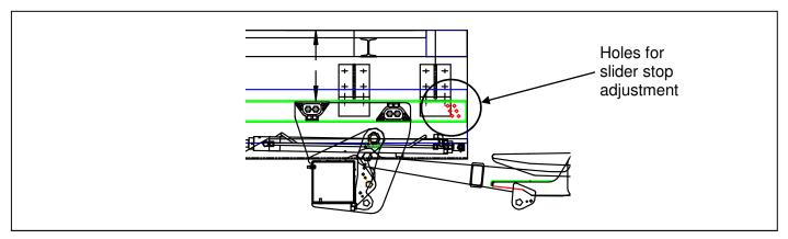
Figure 17 Slider rail stops
