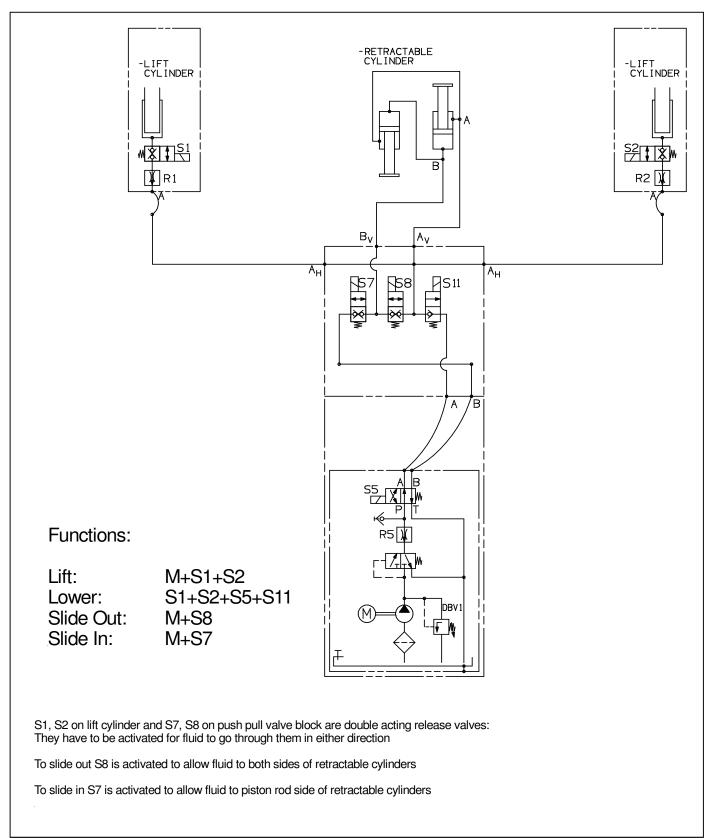
Figure 31 Hydraulic schematic ILFP
