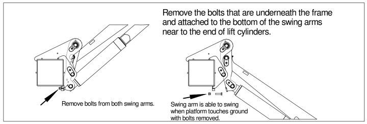
Figure 12 Removal of transportation safety bolts
