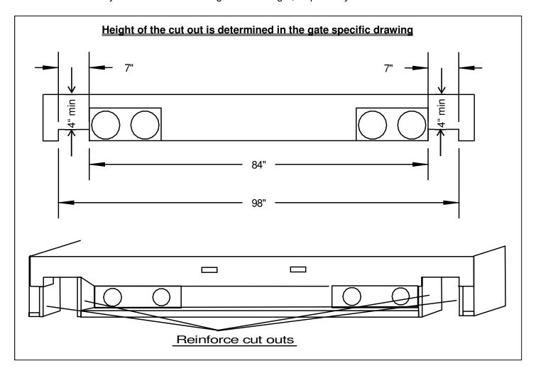
Figure 5 Sill cut-out dimensions - rear view
