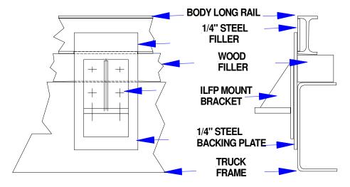
Figure 8 Mount bracket installation details
