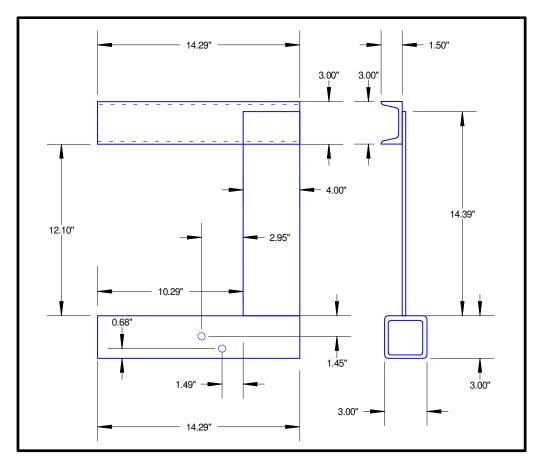
Figure 9 ILFP slide rail mounting fixture
