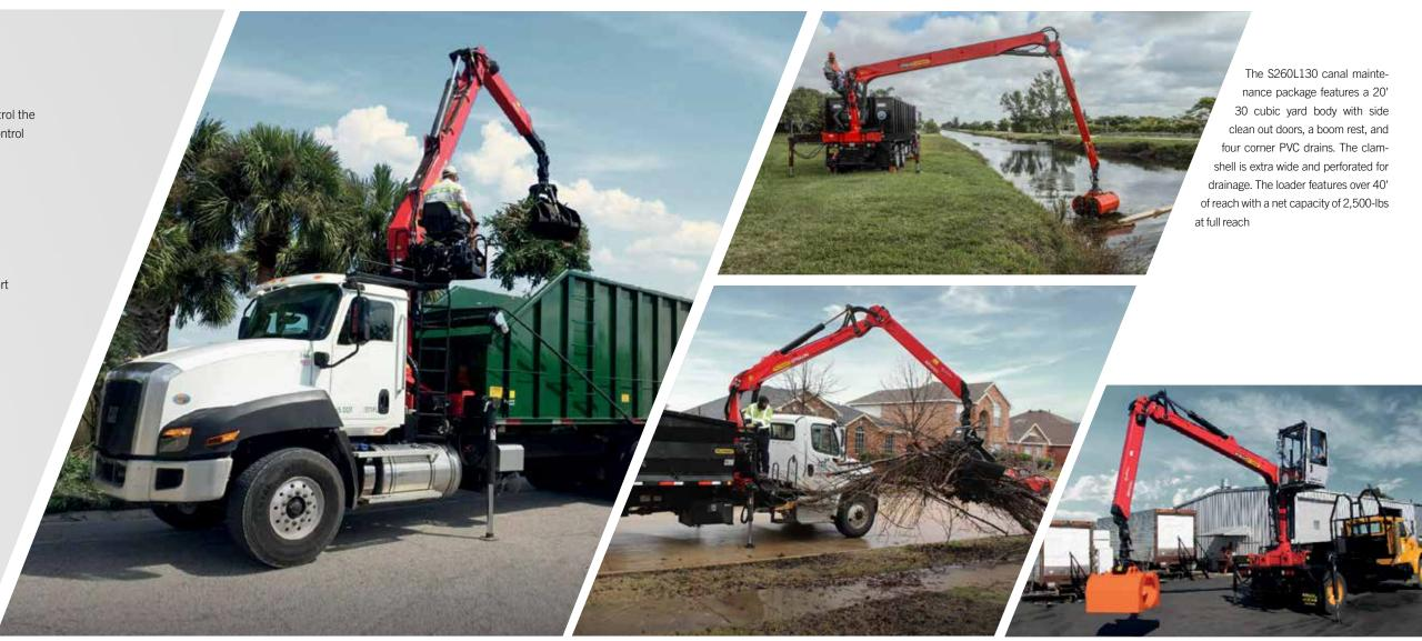
The M110L80 & Q150L80 packages are designed for single or tandem axle trucks. These loaders provide options for longer reaches (32') with higher capacities (3,970-lbs @ 25') and numerous control variations. The out and down stabilizers provide increased stability for those heavy picks.
