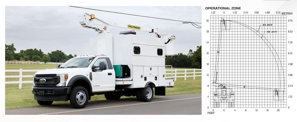
With a 40' working height, 30' side reach, a 24" x 30" bucket, and continuous rotation, the ETT 29 SNT delivers the maneuverability and reach you expect from a PALIFINGER bucket truck. Single-handle control, basket and turret full-pressure hydraulic controls with complete feathering capabilities, an extended shear ball rotation shaft, replaceable pin bushings, an emergency lowering valve, and engine start/stop at the bucket are powerful standard features.
