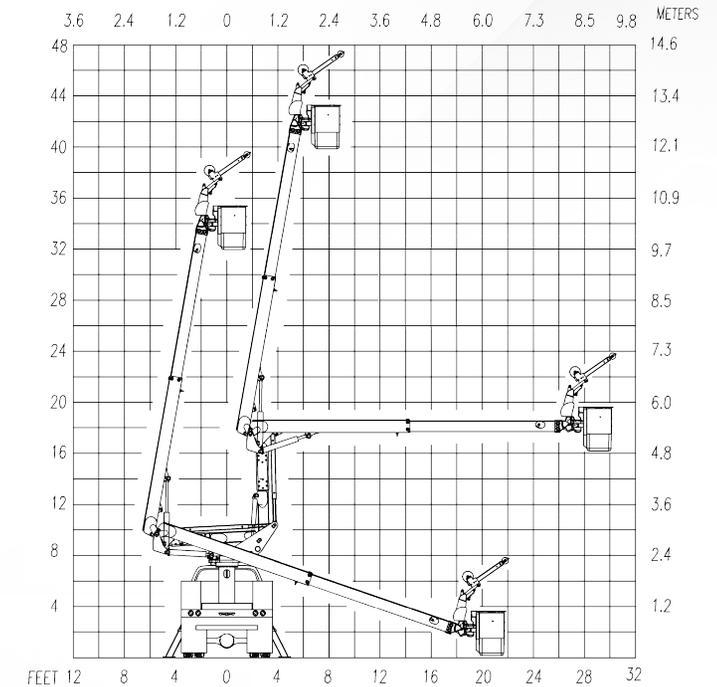
With a 40' working height, 30' side reach, a 24" x 30" bucket, and continuous rotation, the ETC MH 40 IH delivers the maneuverability and reach you expect from a PALFINGER bucket truck. Single-handle control, basket and turret full-pressure hydraulic controls with complete feathering capabilities, an extended shear ball rotation shaft, replaceable pin bushings, an emergency lowering valve, and engine start/stop at the bucket are powerful standard features
