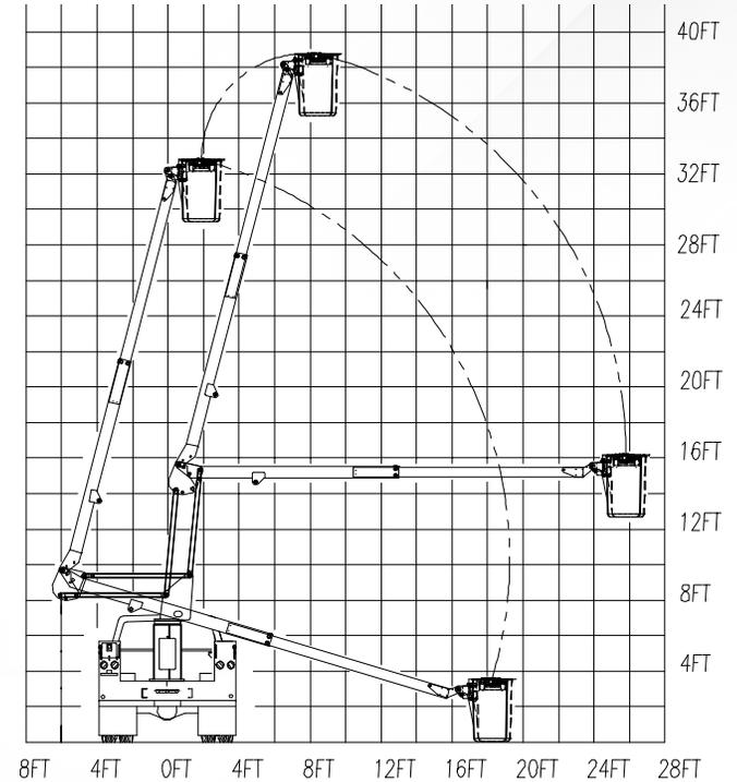
PALFINGER's non-insulated ETC 35 SNT offers standard 390° non-continuous rotation, emergency upper boom-controlled descent, adjustable wear pads, and replaceable bushings for pins. The 350 lbs. capacity bucket also features engine start/stop, hydraulic leveling, an extended gear-drive shaft for manual rotation, and variable speed controls.
