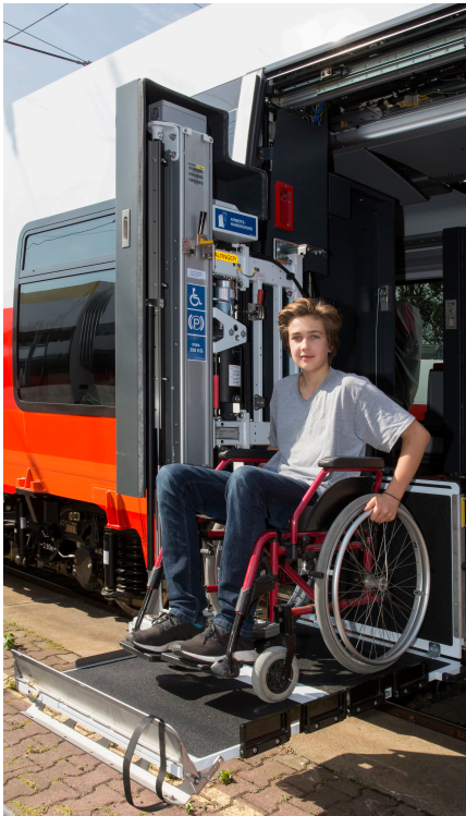
ROTATIONAL LIFT TR Fully hidden behind cover parts
