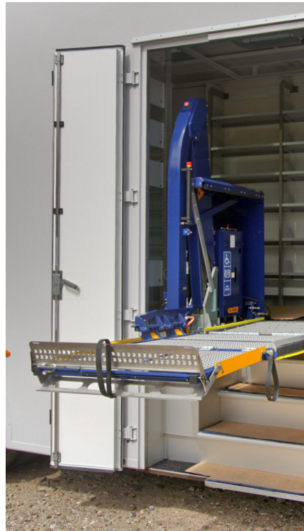
VERTICAL LIFT TRV1 One-arm cover and lift integrated in one solution
