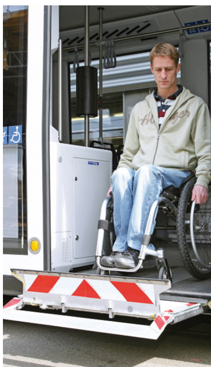
COLUMN LIFT FOR TRAMS SB 300
