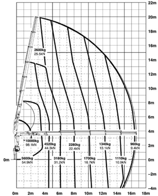
The outreaches stated are with a boom angle of 20° and are therefore not the maximum.
