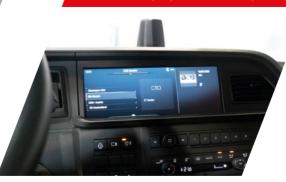
The MAN infotainment system with a high-resolution 12.3-inch color display offers all the high-end features of a modern radio, navigation, and entertainment system. The integration of the rearview camera into this system eliminates the need for an additional dashboard screen.
