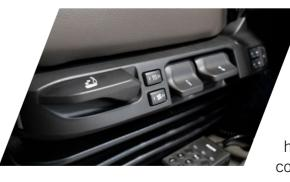
The air-suspended driver-comfort seat with lumbar support, shoulder adjustment, and integrated headrest offers a nine-stage, weight-dependent seat height adjustment. The memory and quick lowering function ensure comfortable entry and exit. The integrated seat heating and ventilation further enhance driving comfort.
