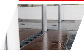
The multitude of tie-down points ensures optimal cargo security. A more customized means of securing all types of cargo is provided by the poles and the integrated bars in the floor. The vehicle is also equipped with container locks, further enhancing flexibility.
