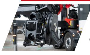
With a variety of available crane attachments that can be easily and ergonomically switched using the specially designed PALFINGER Multifunction Adapter (MFA), this vehicle concept becomes a multifunctional tool perfectly equipped for a wide range of diverse tasks.
