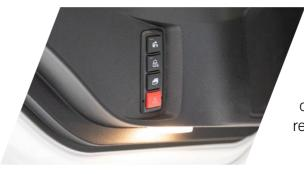
The additional arrangement of four buttons on the driver's door significantly enhances comfort during daily work. This allows important and frequently used vehicle functions to be operated ergonomically without the need to re-enter the vehicle cabin.
