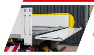
Fold-out brackets at the rear of the vehicle allow the rear wall to be folded down on the same level with the loading platform, eliminating the need to remove it. This extends the loading area and creates an open space to the rear.
