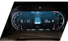
The high-resolution, fully digital Combination Instrument Professional is a 12.3-inch color display. It presents all the essential operational information required for vehicle operation to the driver in a clear and easily comprehensible manner. The fully digital display introduces a new way of visualization with optimal information transfer to the driver.
