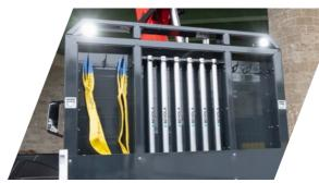
The multifunctional front wall in anthracite color provides multiple storage options for chains, tie-down straps, and round slings using hooks or a dust box, ensuring secure storage during transit. Furthermore, the front board features a pole storage area.
