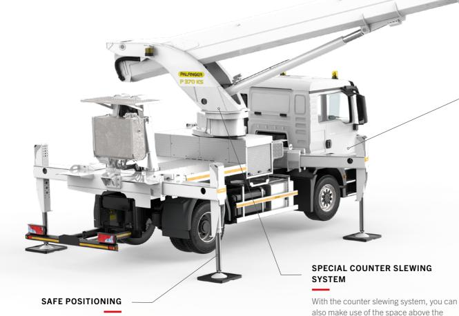
The stabilizers are levelled automatically. With their lift of up to 1000 mm, they can equalize all but the most difficult terrain with ease. The controls for the stabilizers are located on the left and right side of the base.
