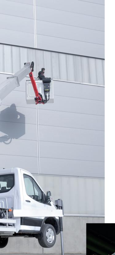
The lightest model in the TEC range offers you the greatest flexibility in configuration and use. Doesn't matter if its an additional battery pack for hybrid operation or different configurations and features, there is space for everything on the PT 19 TJ. This model comes with 19 meter working height, an improved 13.9 m maximum outreach and 300 kg basket load. Take your efficiency to the next level thanks to improved ergonomics, better stability and a wide variation of possible chassis.
