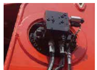
Two Speed Winch
