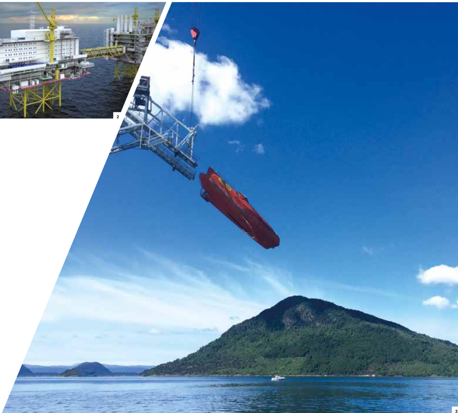
1. Nine free-fall lifeboat systems in one structure | 2. Johan Sverdrup living quarters (© Statoil ASA) | 3. Free-fall testing
