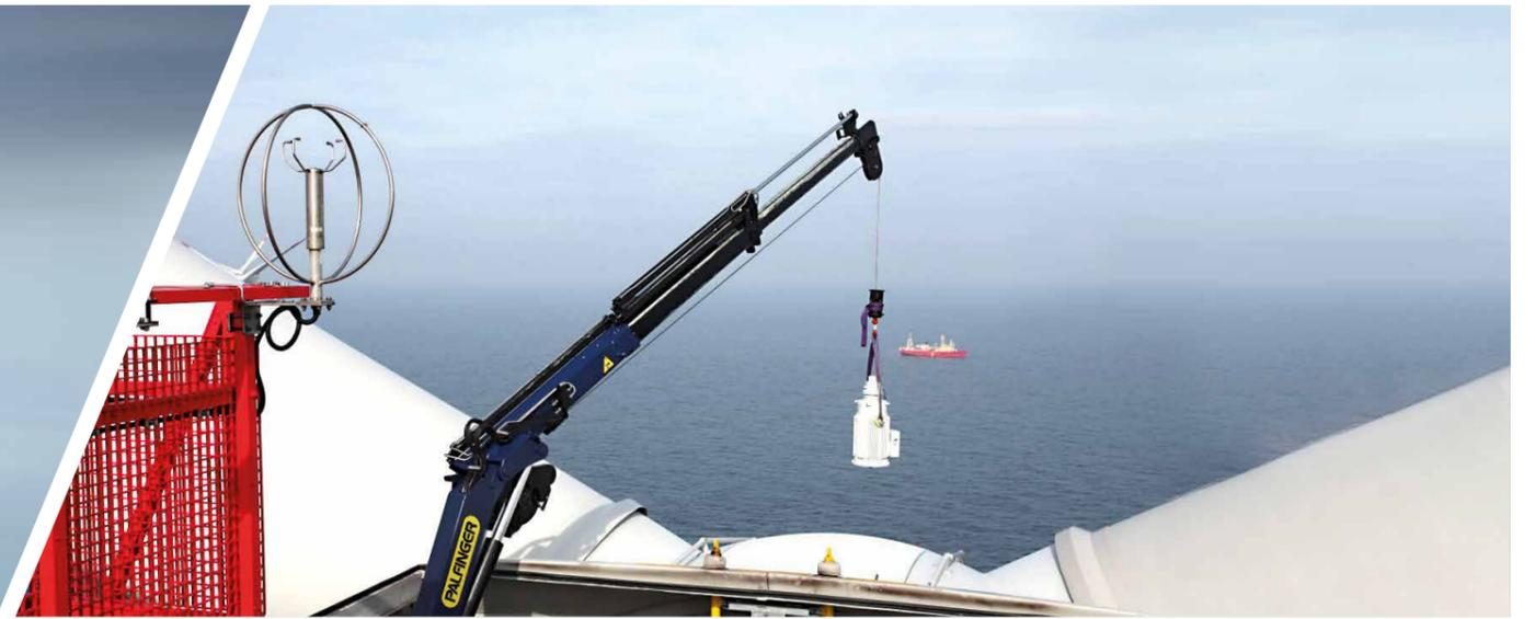
Work can be undertaken quickly and easily using PALFINGER MARINE's nacelle cranes.
