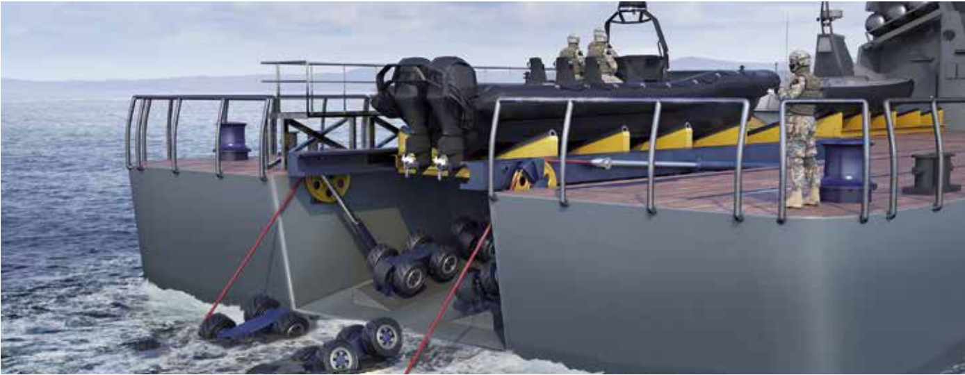
Quad wheel drive units mounted on foldable stern ramp and on deck structure.
