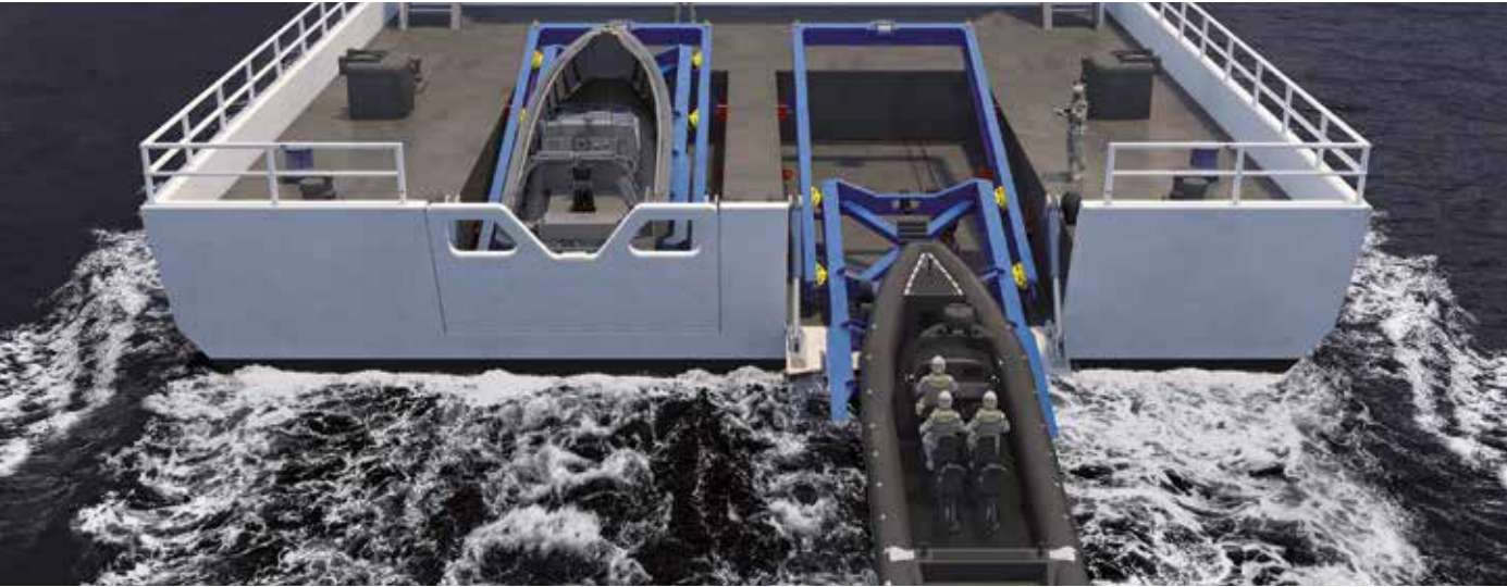
Drive-able slipway frame (In/Out)
