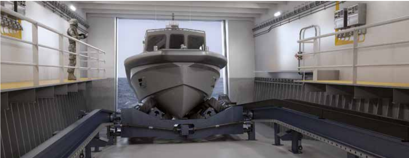
Drive mechanism for slipway frame
