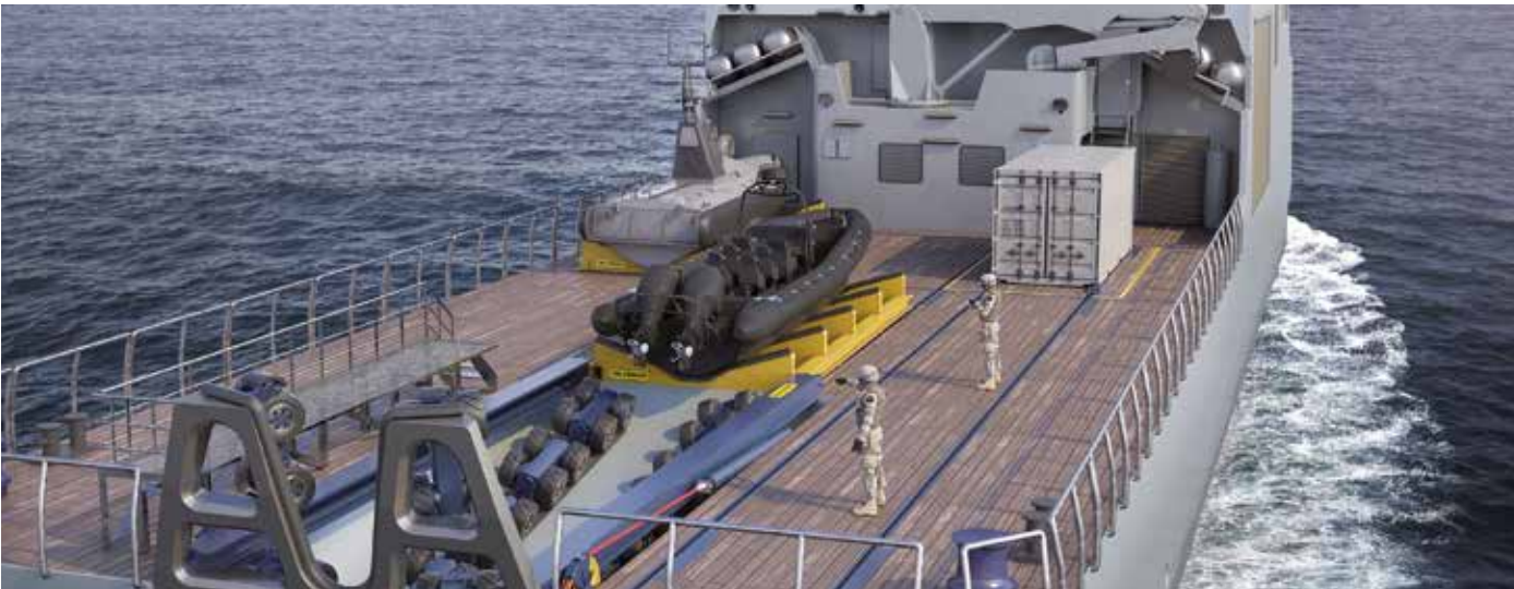
Boat parking cradles for wide beam boats and narrow beam boats
