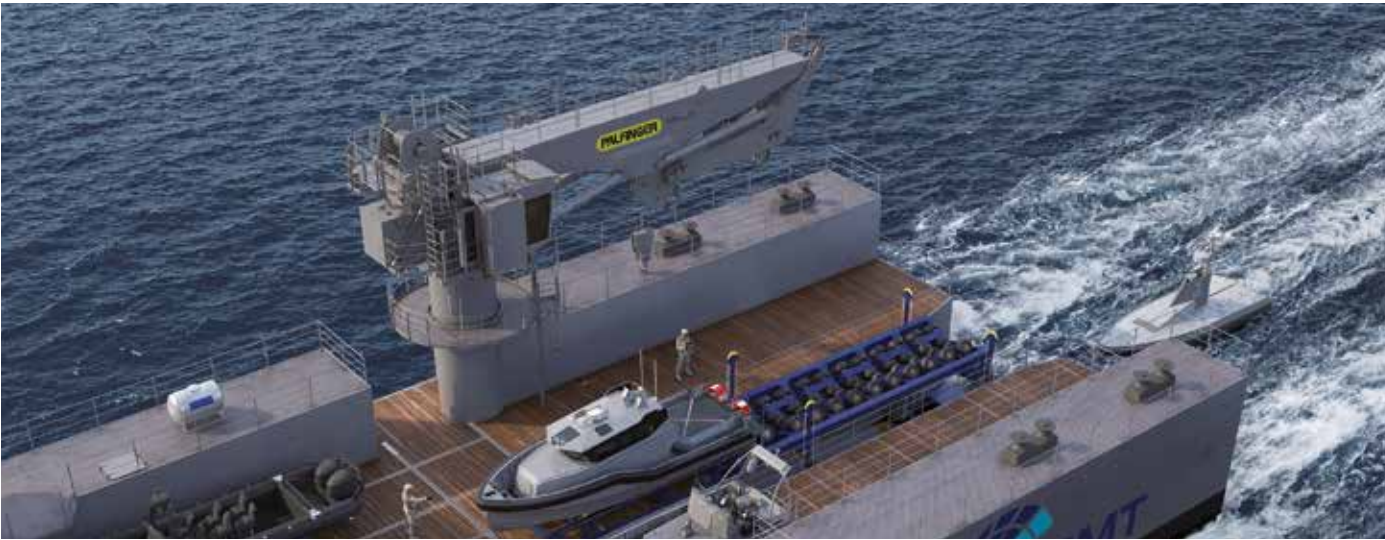
Slipway frame elevator; Extendable boat transfer unit
