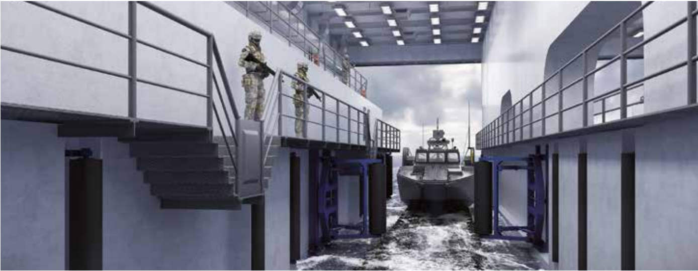
Buffer devices for each boat parking position
