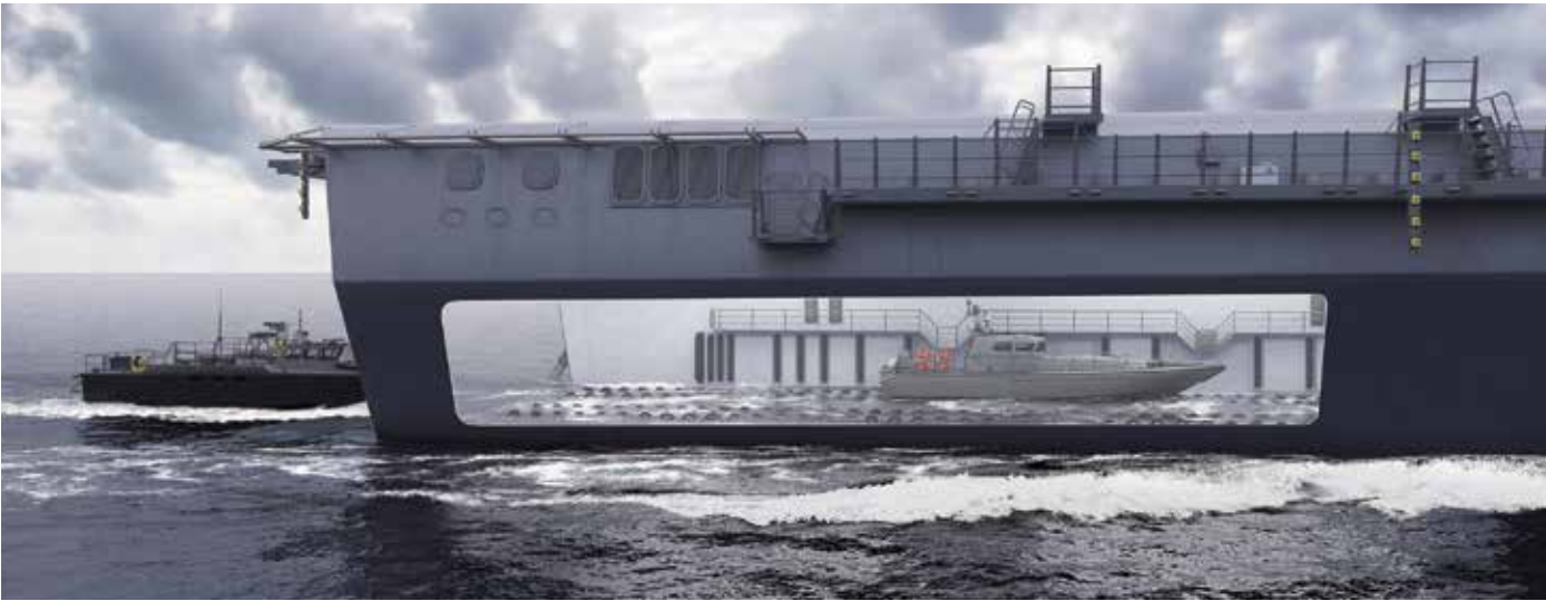
Submergible slipway slopes (by ballasting vessel down)
