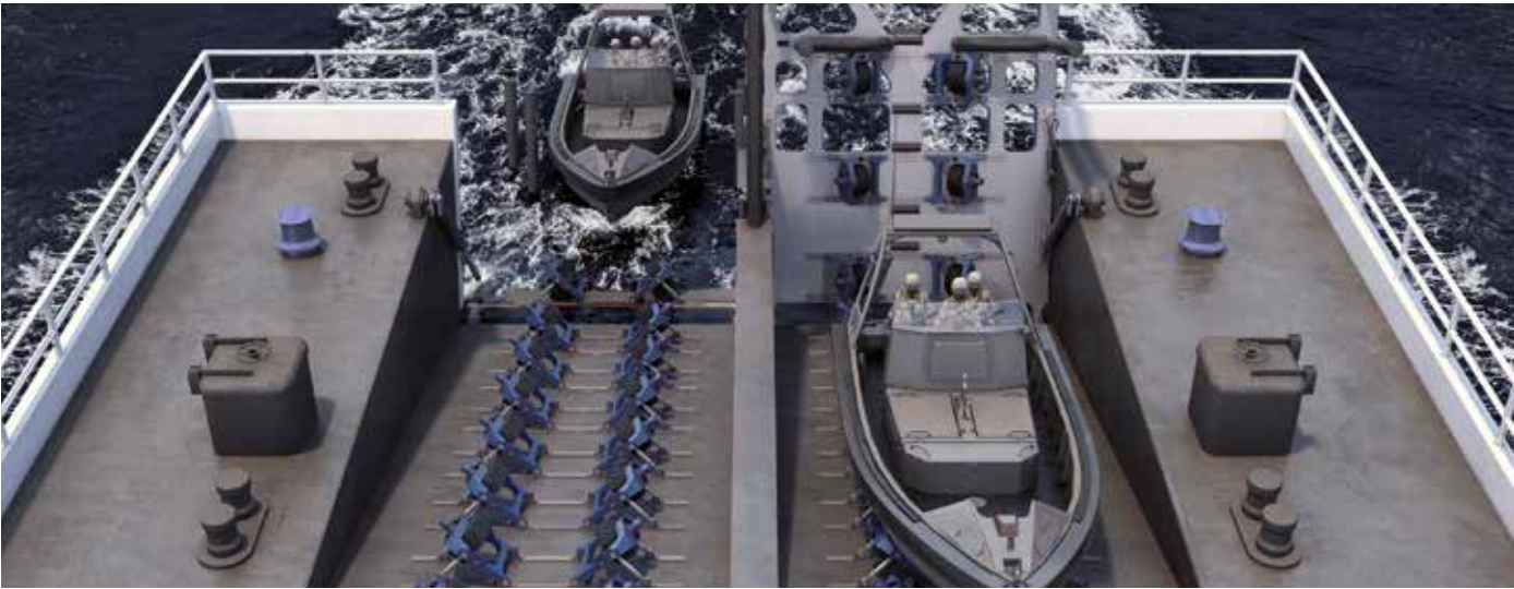
Stern ramp with single wheel drive units
