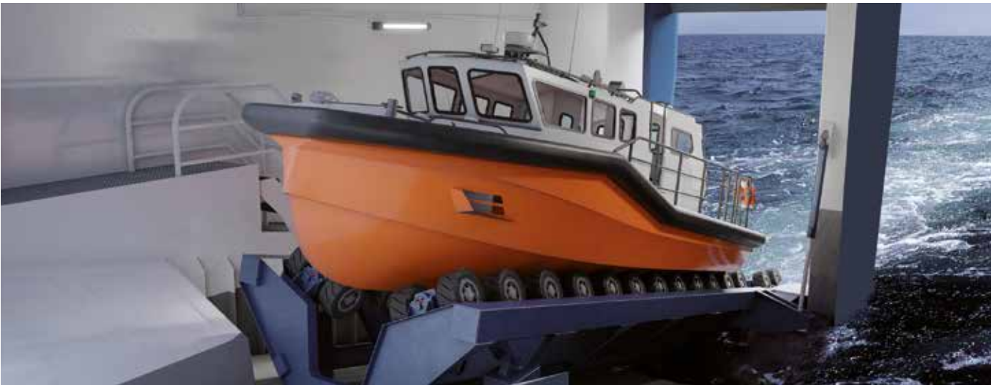
Two submerged wheel units on vessel transom
