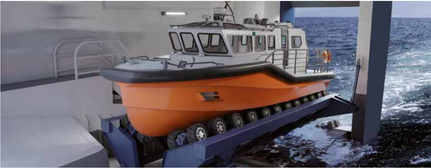
Quad wheel drive units mounted on slipway frame
