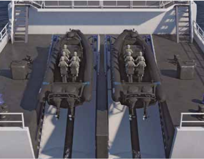
Extendable and retractable boat cradle - Double
