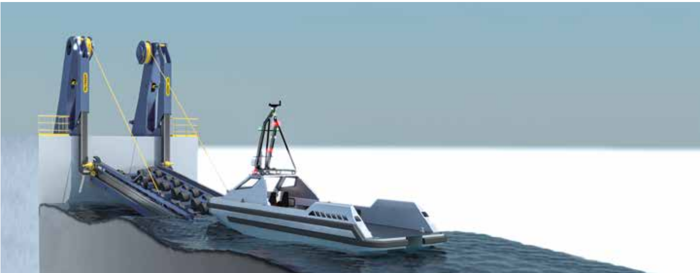
PQBS-D-C Slipway system lowered to optimal launch and recovery angle
