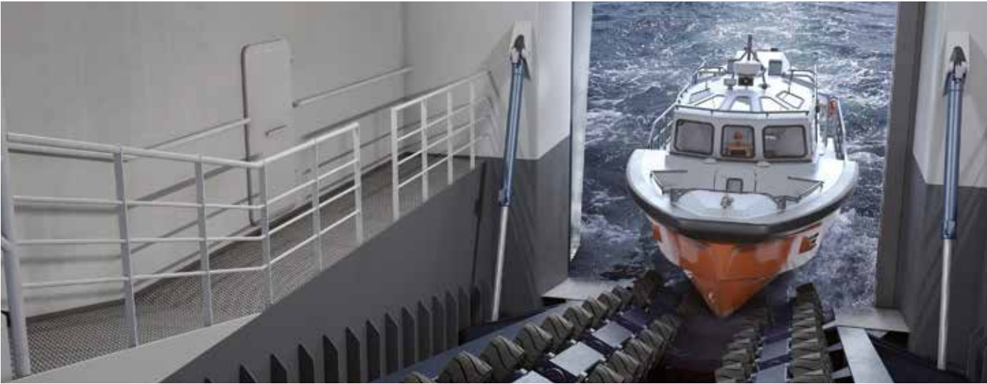
Tilting mechanism for slipway frame
