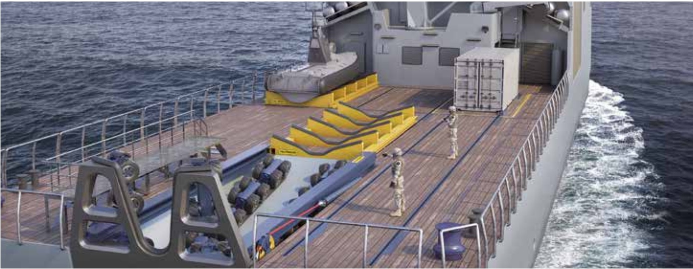
Boat cradle elevator and skidding system for boat cradles
