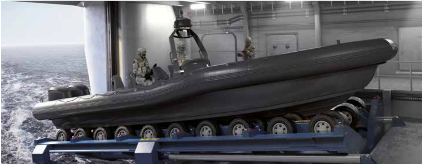
Mechanism for extension and retraction of slipway frame
