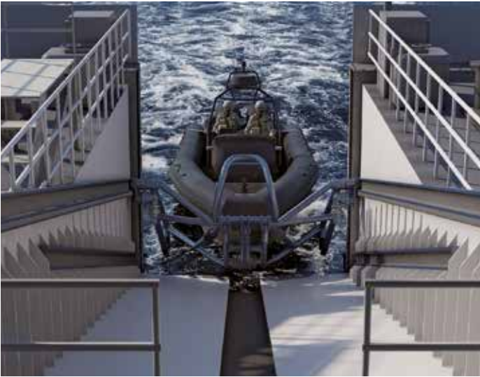
Asymmetric drive and guide rails
