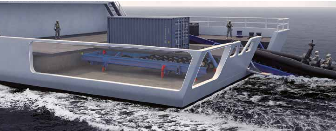
Slipway frame stowed and secured below hatch cover. Container on top of hatch cover.
