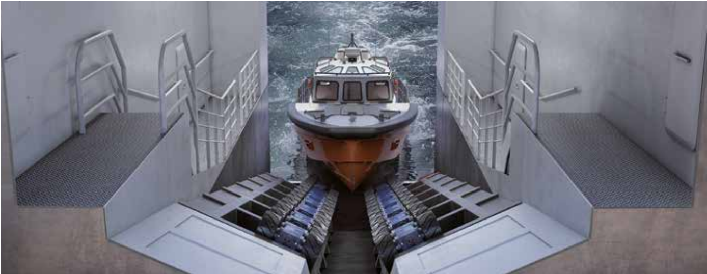
Slipway with 12° slope angle
