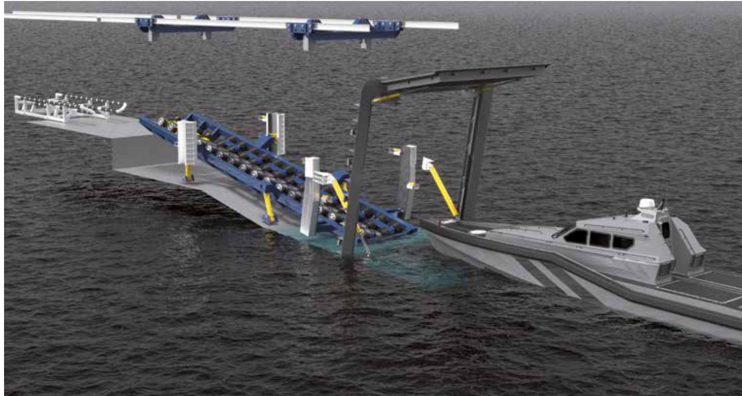
Quad wheel-drive units mounted on foldable stern door/ramp and on slipway cradle.
