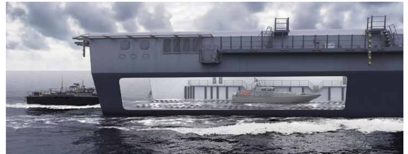
Submersible slipway slopes (by ballasting vessel down)
