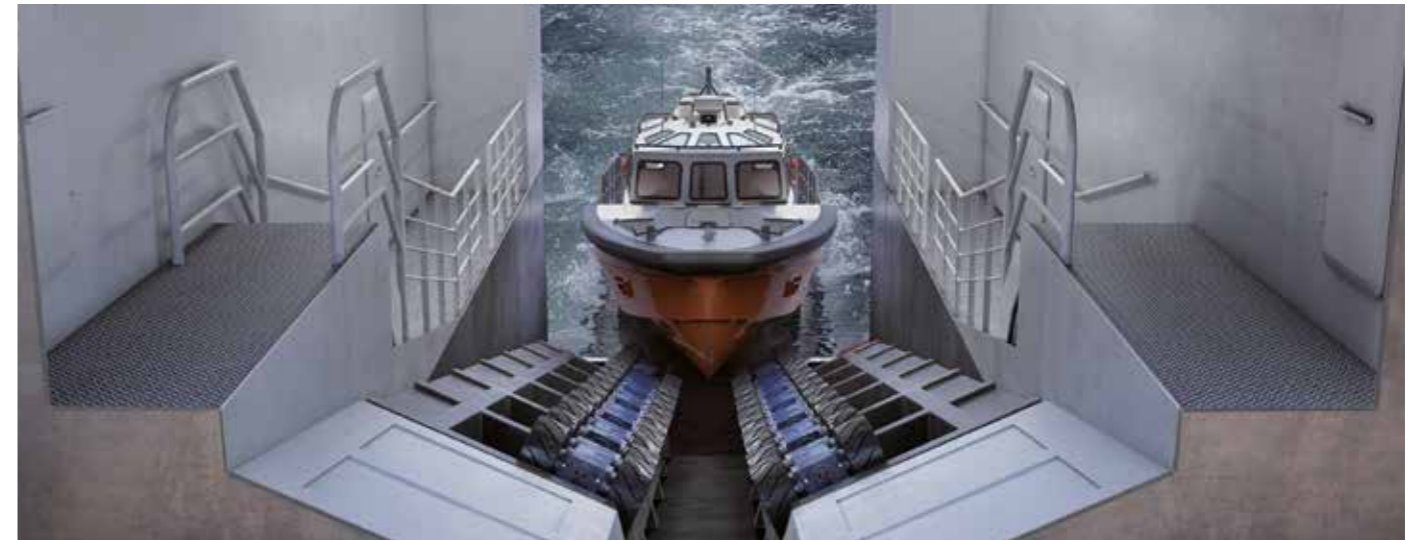
Slipway with 12° slope angle
