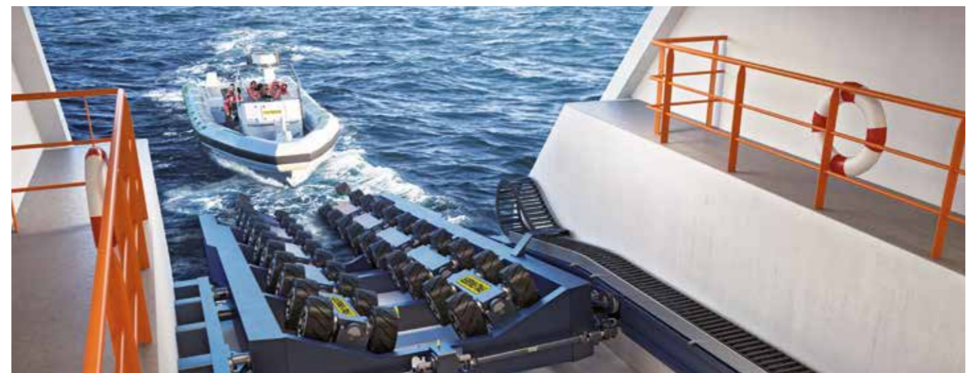
Rack & pinion drive mechanism for slipway cradle
