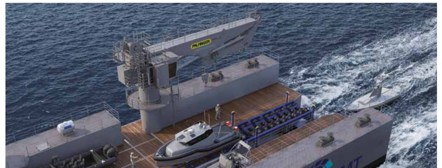
Slipway cradle elevator; Extendable boat transfer unit
