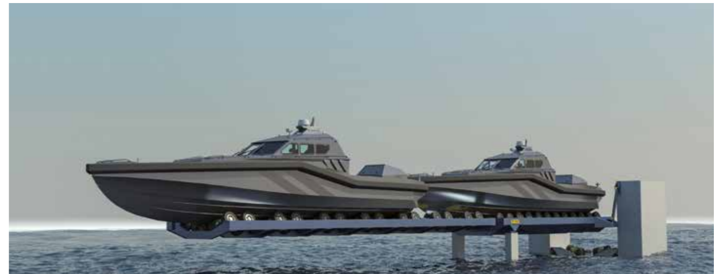
Boat #1 in parking position on parking cradle and boat #2 in launch/recovery position on slipway cradle
