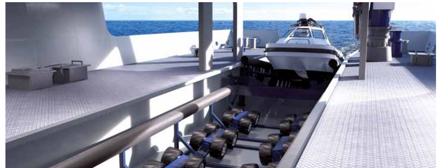
Slipway frame and deployable cradle at launch/recovery angle. Powered parking cradle in front of tiltable slipway frame for transfer of boat to/from the deployable slipway cradle
