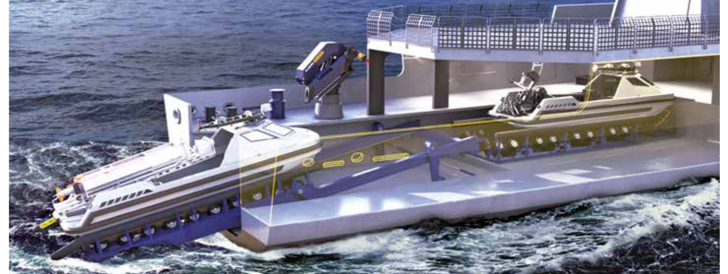
Submerged guide rails and drive wheel units on deployable slipway cradle, supported by tiltable slipway frame
