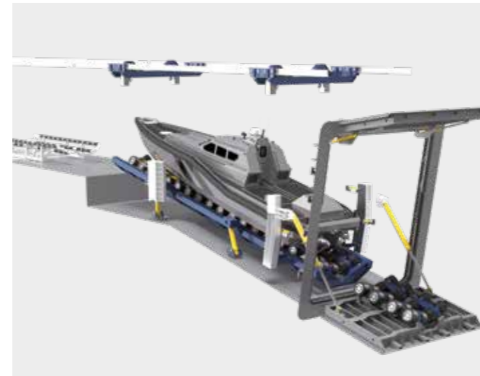
Slipway cradle in launch/recovery position
