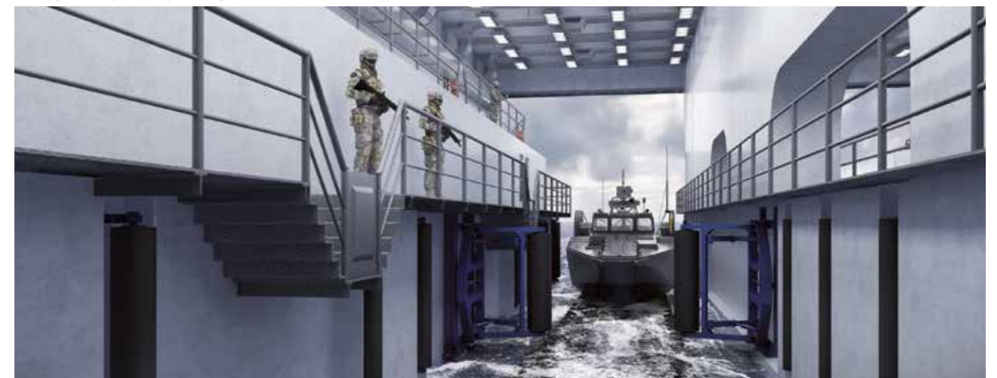
Buffer devices for each boat parking position
