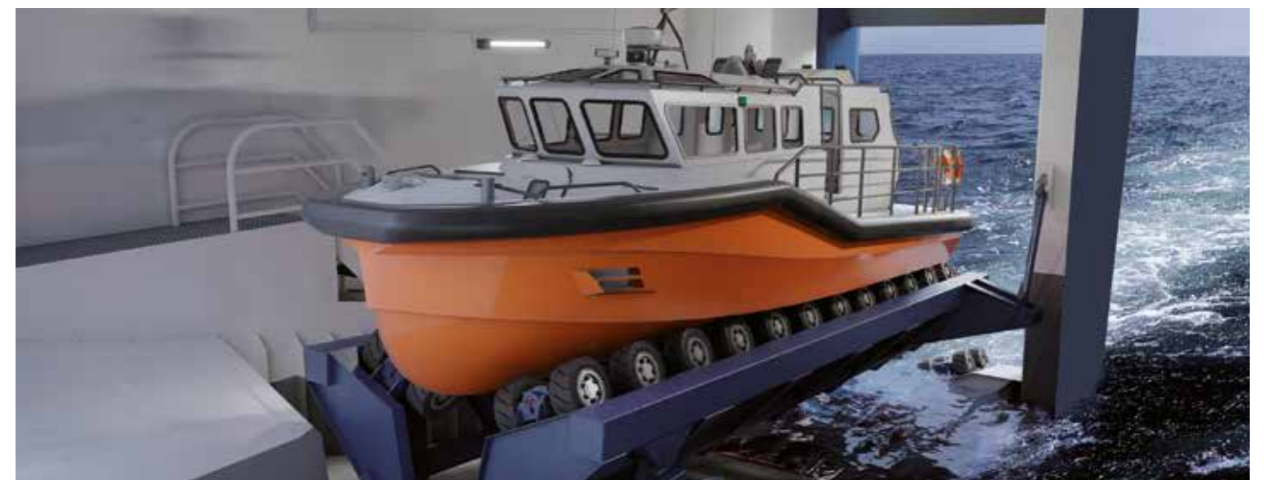
Hydraulic operated tilt-mechanism for slipway cradle
