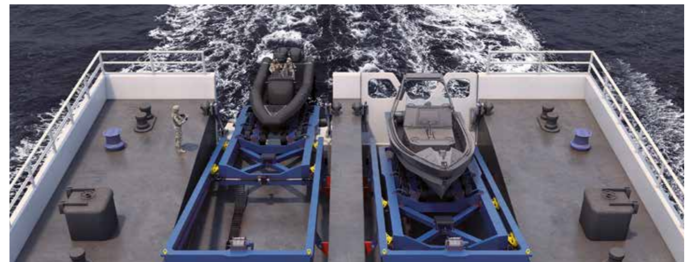
Quad wheel-drive units mounted on slipway cradle
