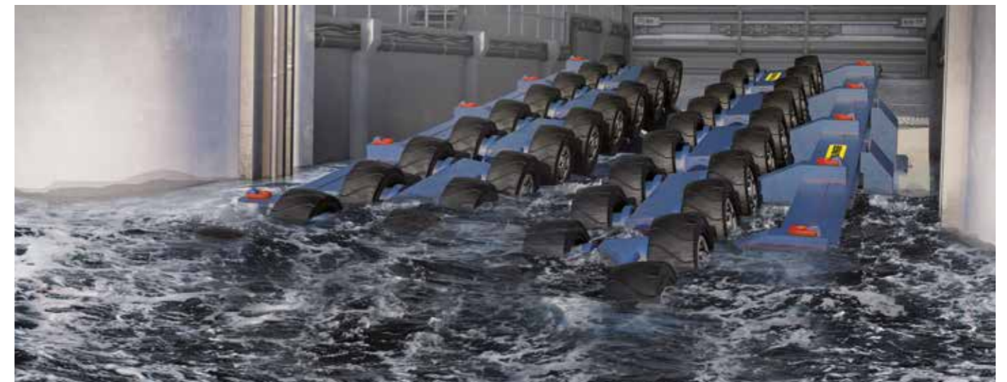
Quad wheel-drive units mounted on slipway cradle
