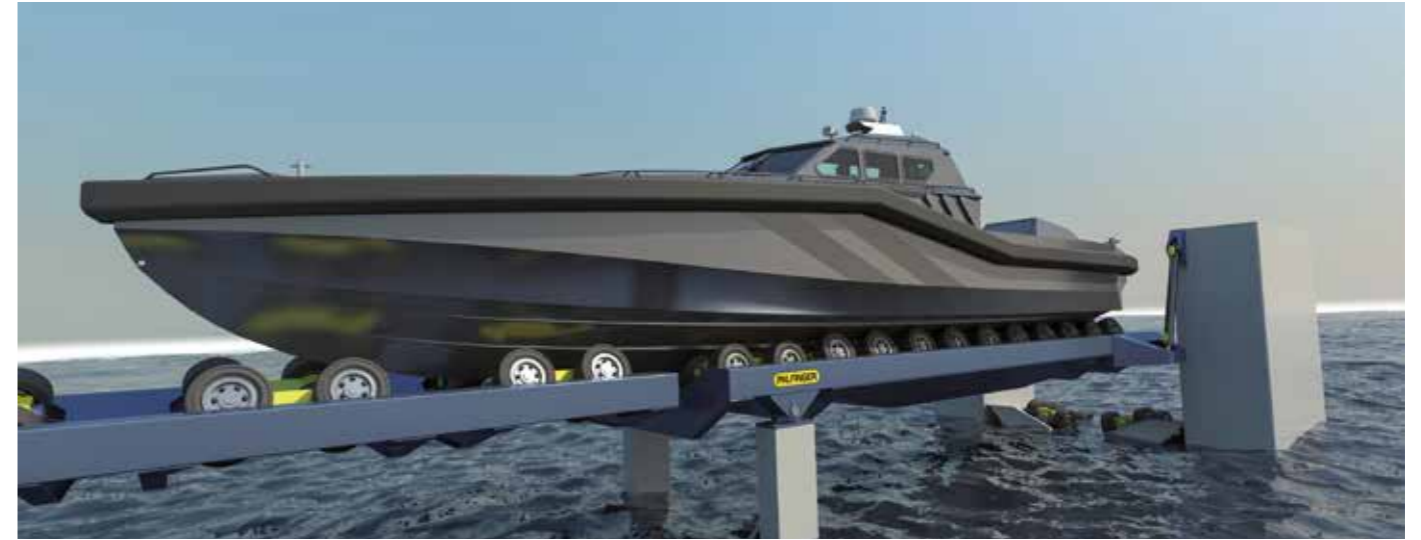
Boat #1 in elevated position on slipway cradle
