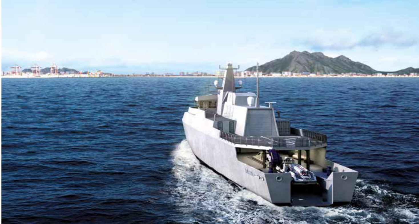
Cybele 90m MCMV vessel design and ARCIMS Modular USV system, used with permission from Babcock International and ATLAS ELEKTRONIK UK Ltd.
