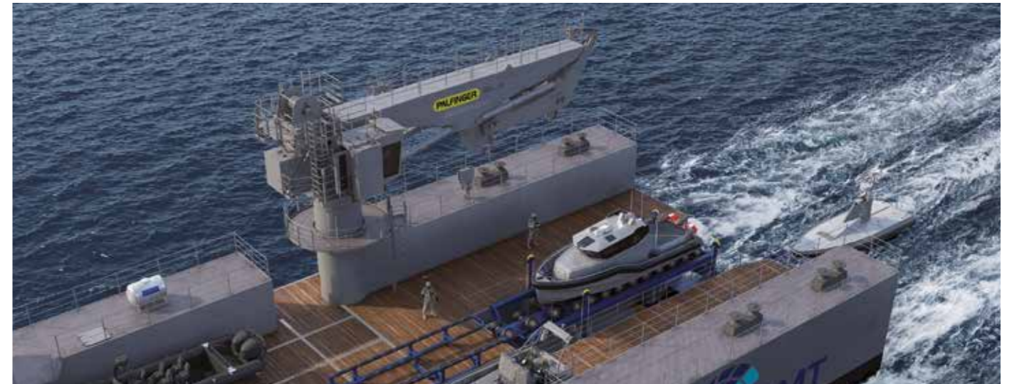
Slipway cradle elevator; Extendable boat transfer unit
