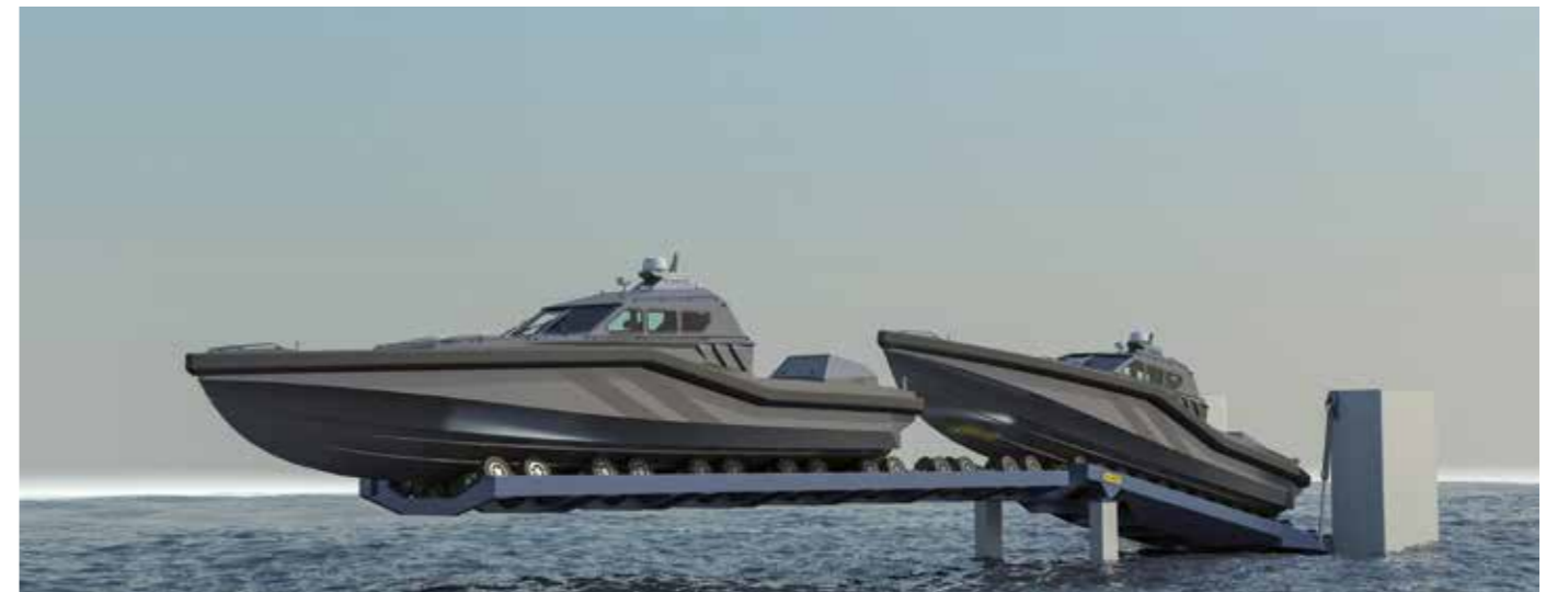
Boat #1 in parking position on parking cradle and boat #2 in elevated parking position on slipway cradle
