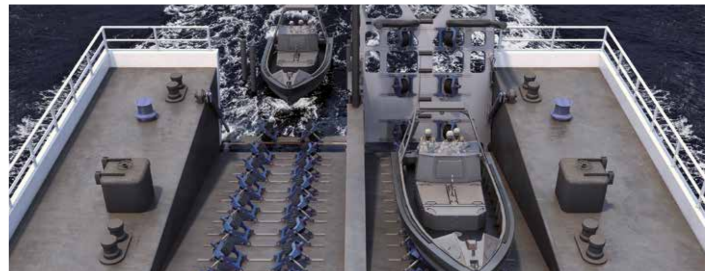
Stern ramp with single wheel-drive units
