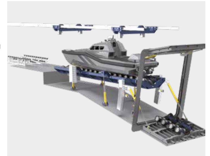
Slipway cradle in elevated position
