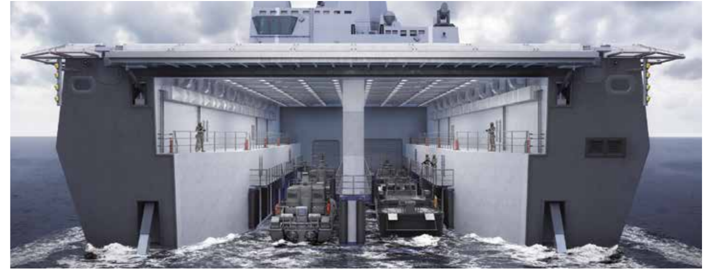
Quad wheel-drive units on deck structure in mission bay
