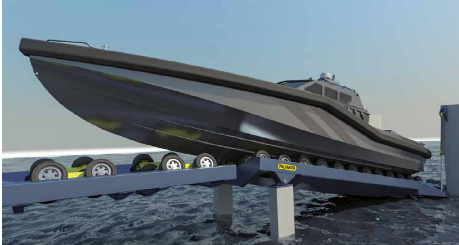
Boat #1 in launch/recovery position on slipway cradle
