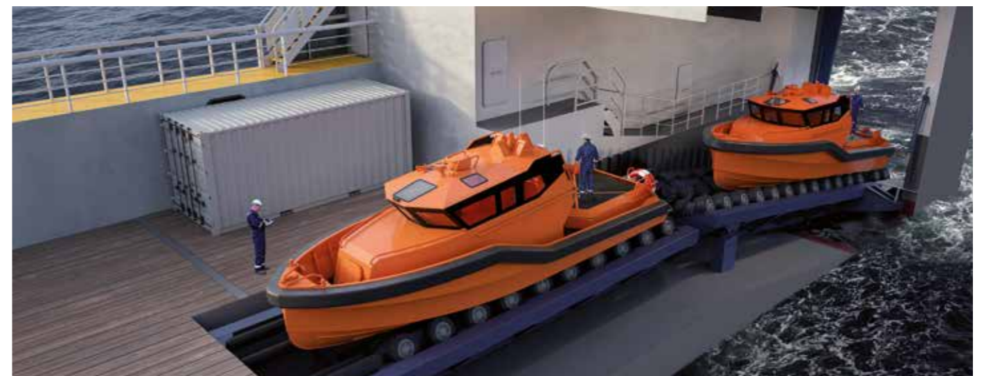
Slipway cradle in launch and recovery position
