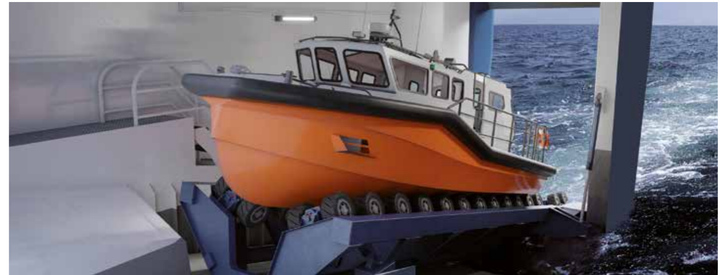
Slipway cradle with quad wheel-drive units
