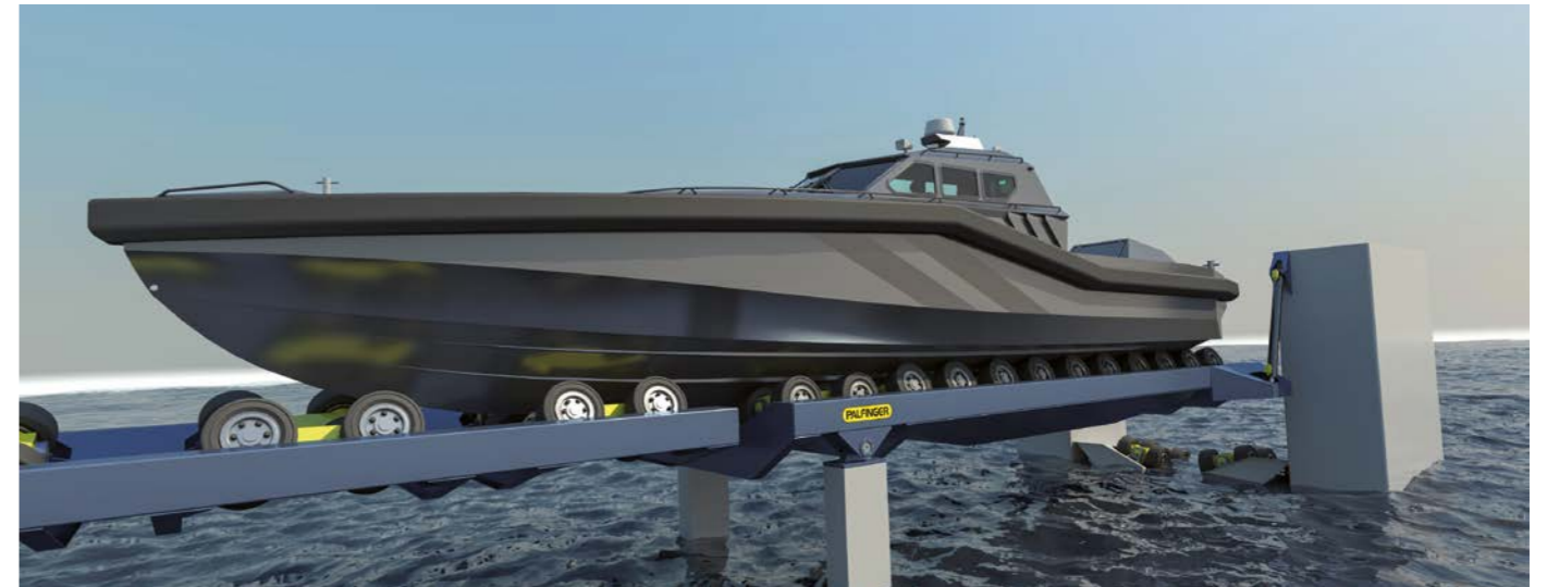
Boat #1 in elevated position on slipway cradle
