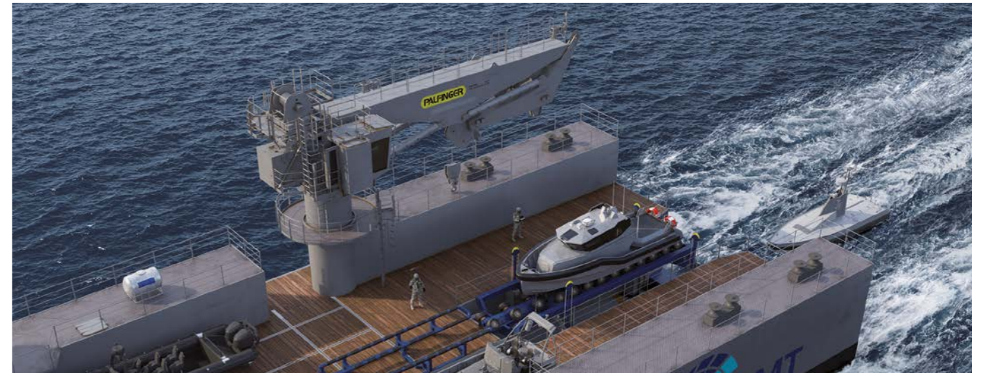
Slipway cradle elevator; Extendable boat transfer unit
