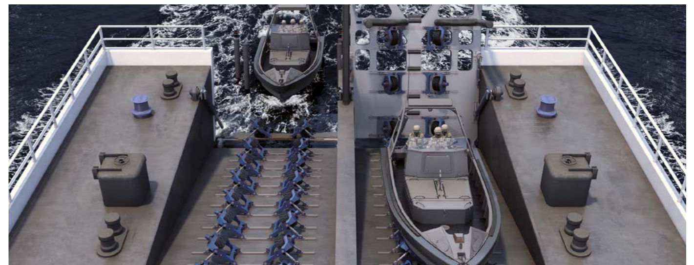
Stern ramp with single wheel-drive units
