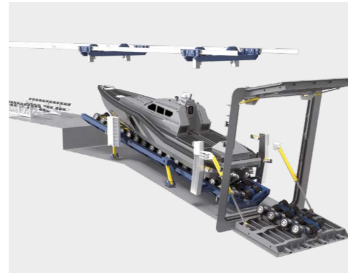
Slipway cradle in launch/recovery position
