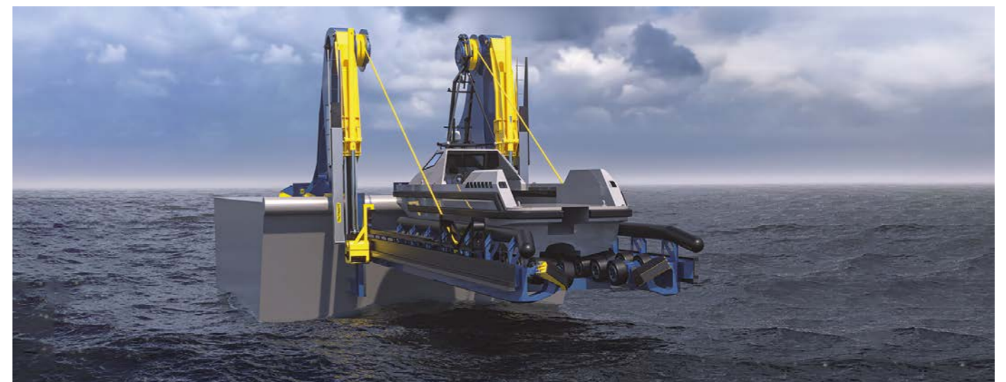
Slipway cradle lowered to optimal launch and recovery height
