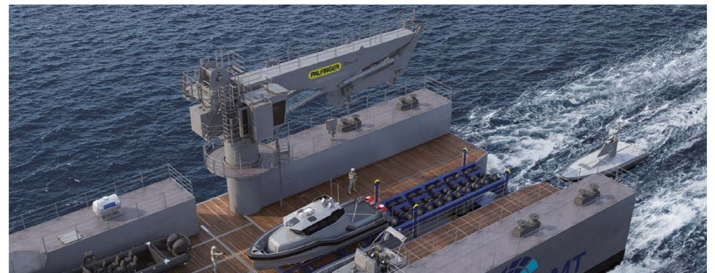
Slipway cradle elevator; Extendable boat transfer unit
