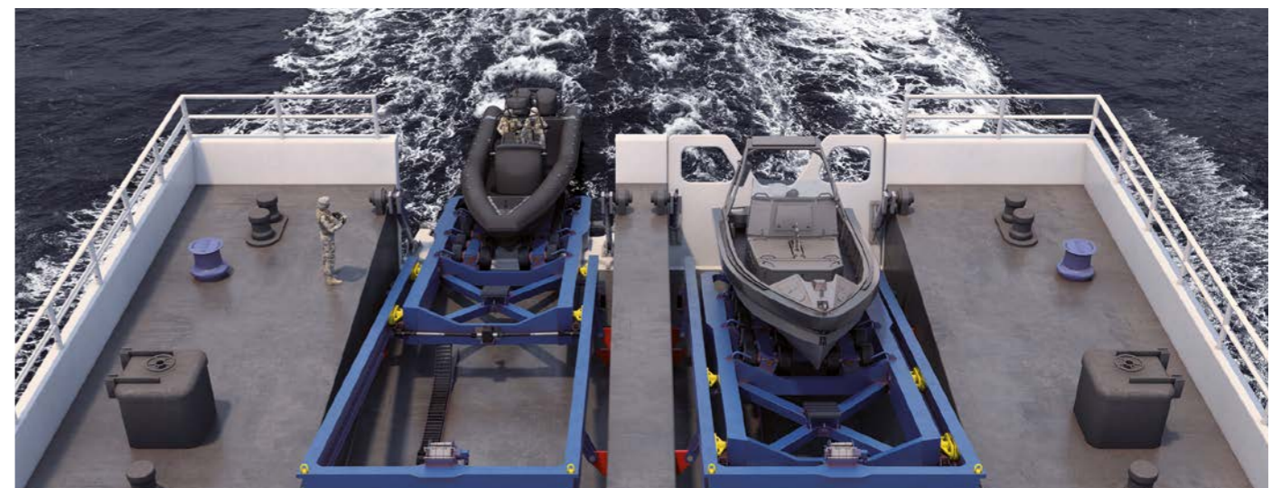
Quad wheel-drive units mounted on slipway cradle
