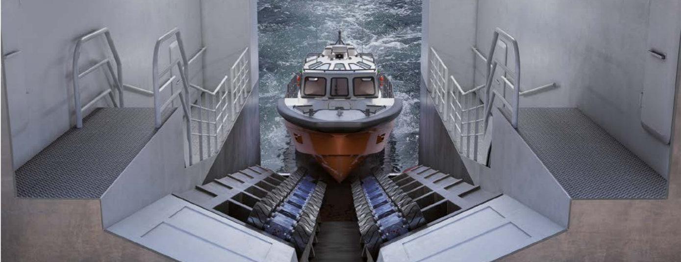
Slipway with 12° slope angle
