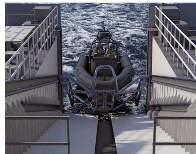
Asymmetric drive and guide rails
