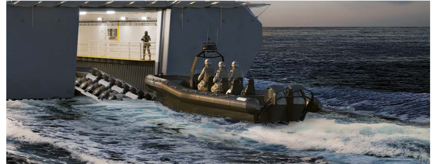
Slipway cradle in launch and recovery position
