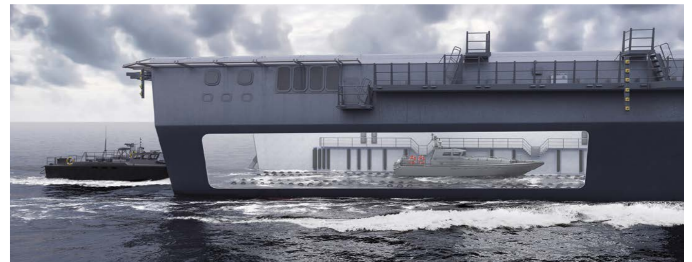
Submergible slipway slopes (by ballasting vessel down)
