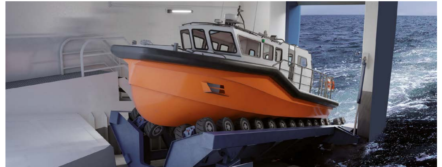
Slipway cradle with quad wheel-drive units
