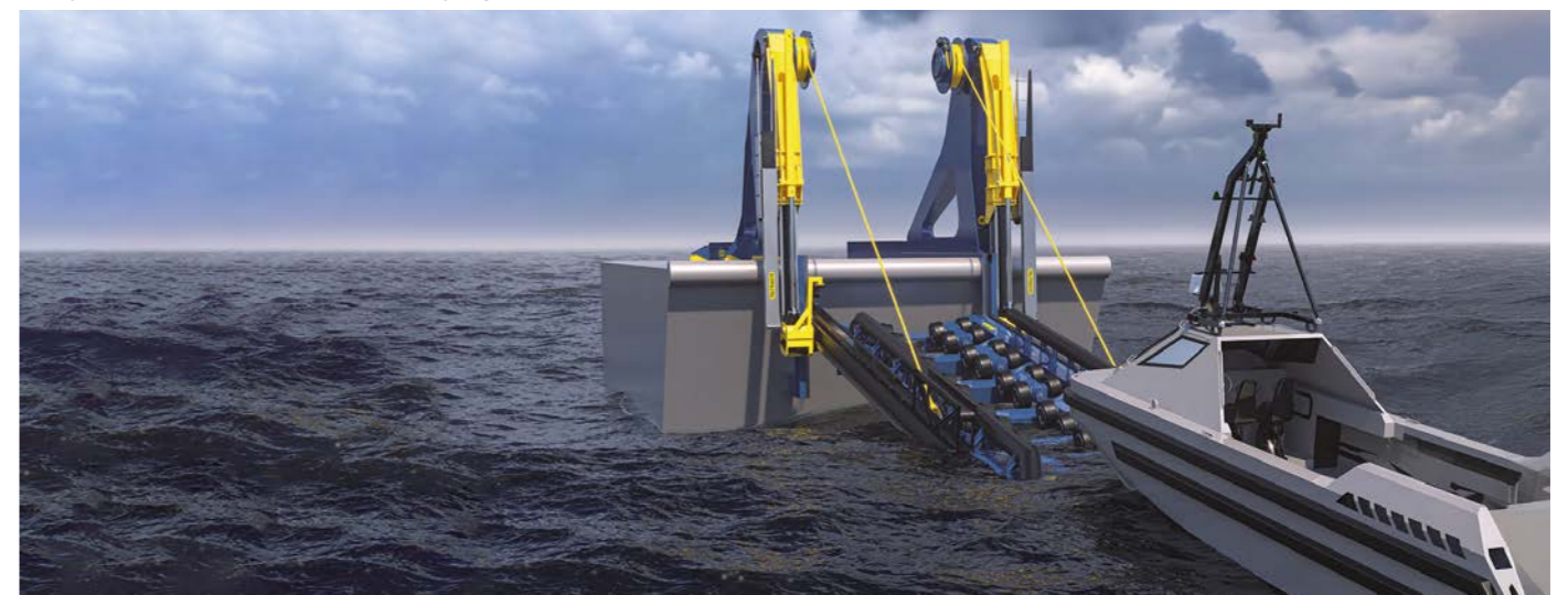
Slipway cradle lowered to optimal launch and recovery angle
