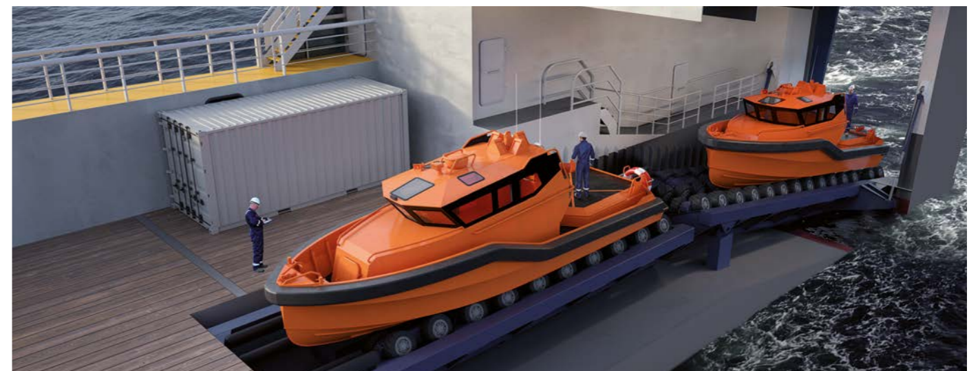
Slipway cradle in launch and recovery position
