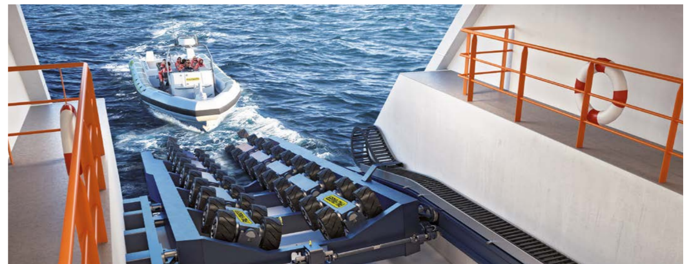
Rack & pinion drive mechanism for slipway cradle
