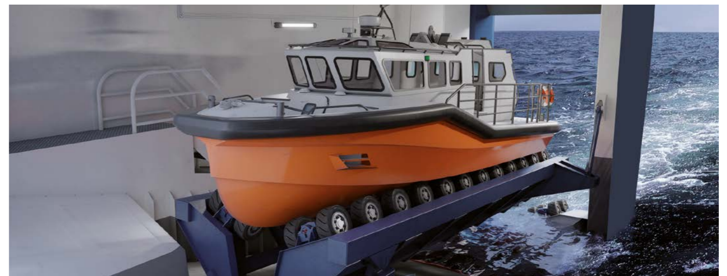
Hydraulic operated tilt-mechanism for slipway cradle
