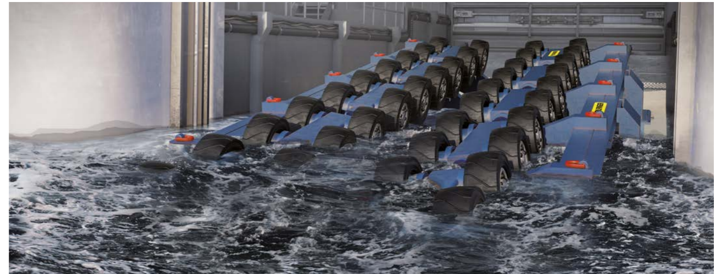
Quad wheel-drive units mounted on slipway cradle
