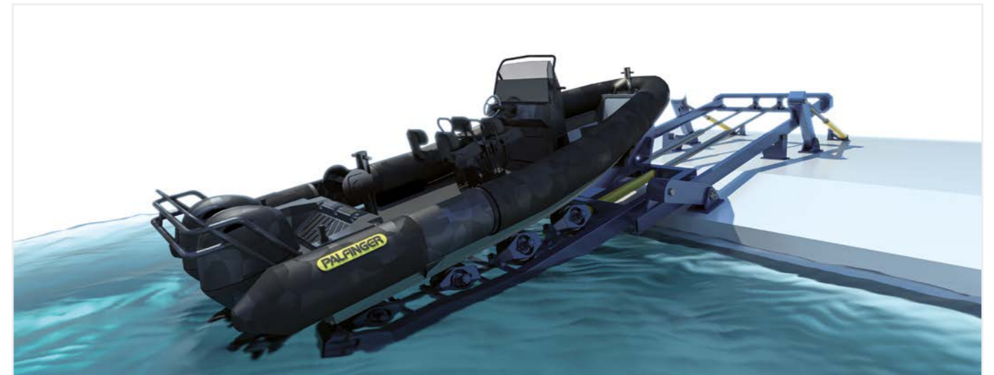
Boat with twin outboard engines, fully recovered into the extended slipway cradle
