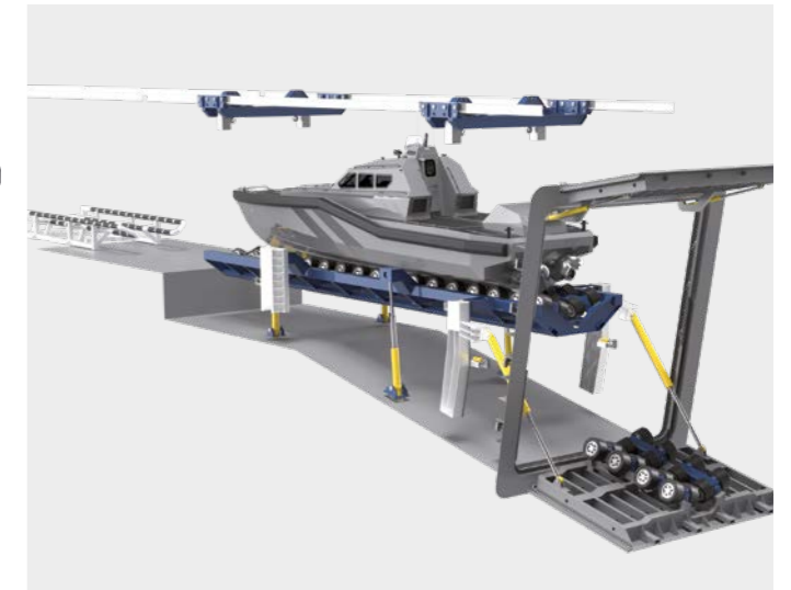
Slipway cradle in elevated position
