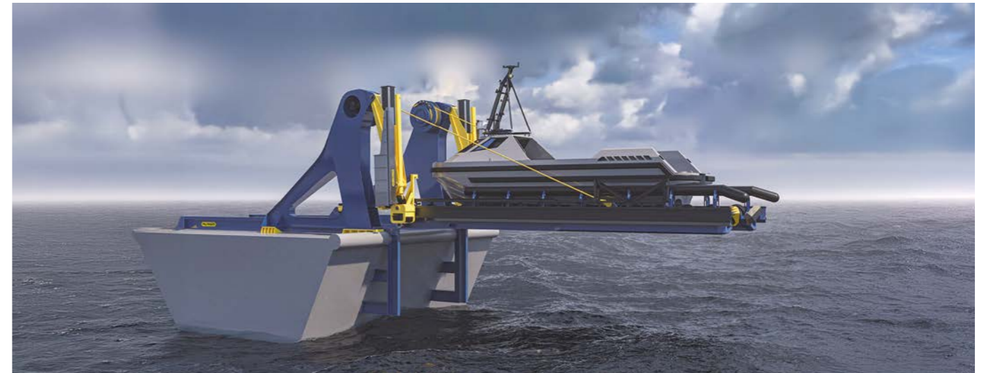
Slipway cradle in outboard transition position
