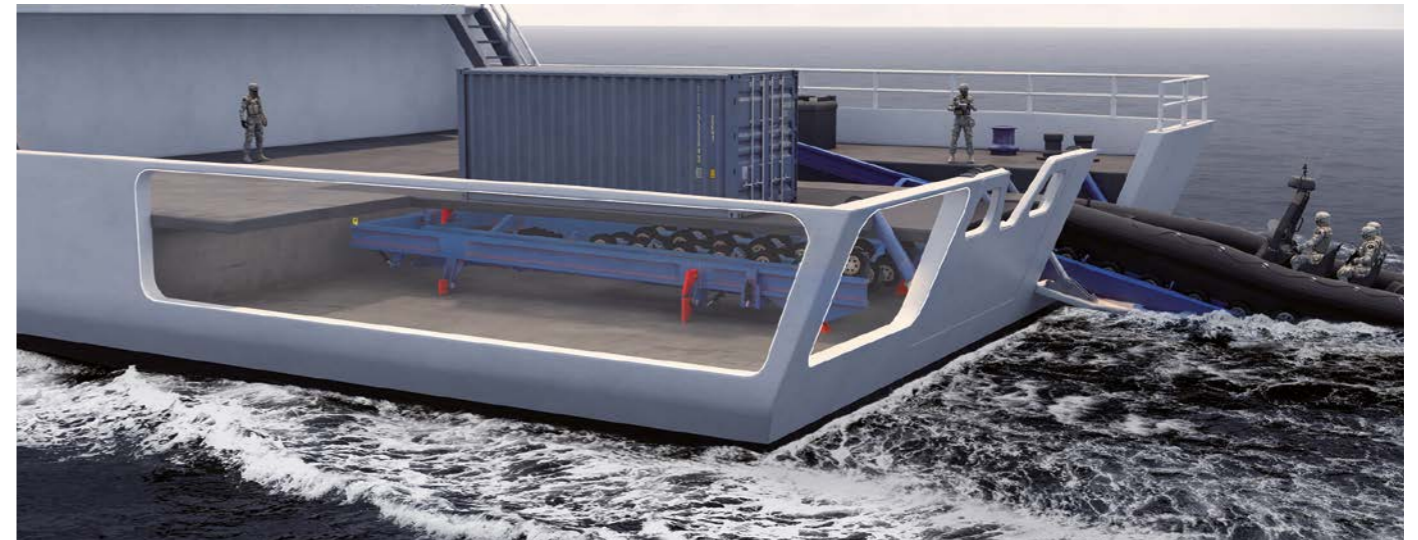
Slipway cradle stowed and secured below hatch cover. Container on top of hatch cover.
