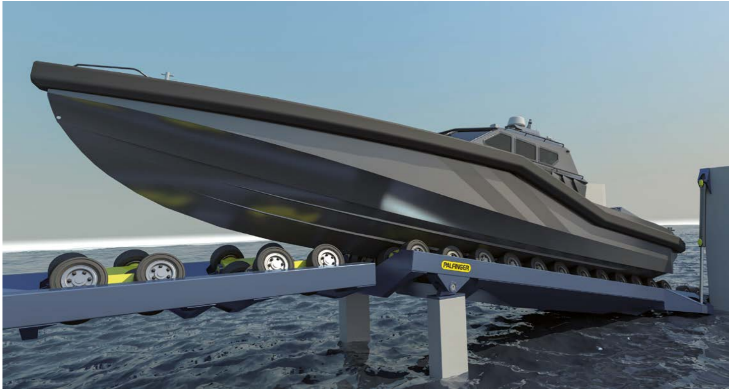
Boat #1 in launch/recovery position on slipway cradle
