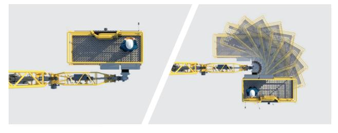
The OPTS is controlled from the hardwired remote-control unit on deck or from the control station on the basket.
