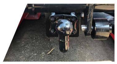
**Ballhead coupling** for VAN and VAN FLEX
