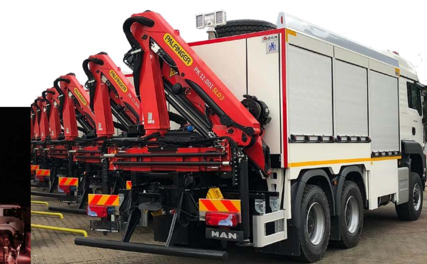
with tried-and-trusted PALFINGER quality proved essential in AFAD's decision to place this major order. In combination with the wide range of equipment on offer, the PK 11.001 SLD 3 from the medium crane range is a real all-rounder for a diverse array of applications.
