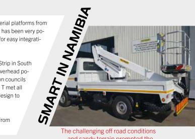
and sandy terrain prompted the need for a compact and robust combination and thus the customer opted for the P 140 T fitted onto a 4X4 supplied by Erongo Commercial Vehicles, the local lveco dealer in Namibia.
