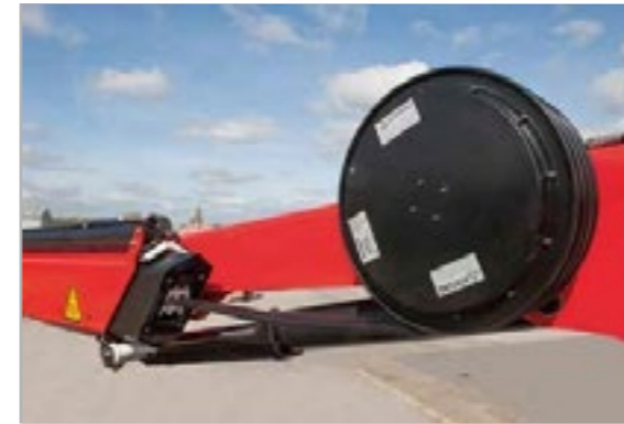
Additional hose equipment on extension booms CODE 4
