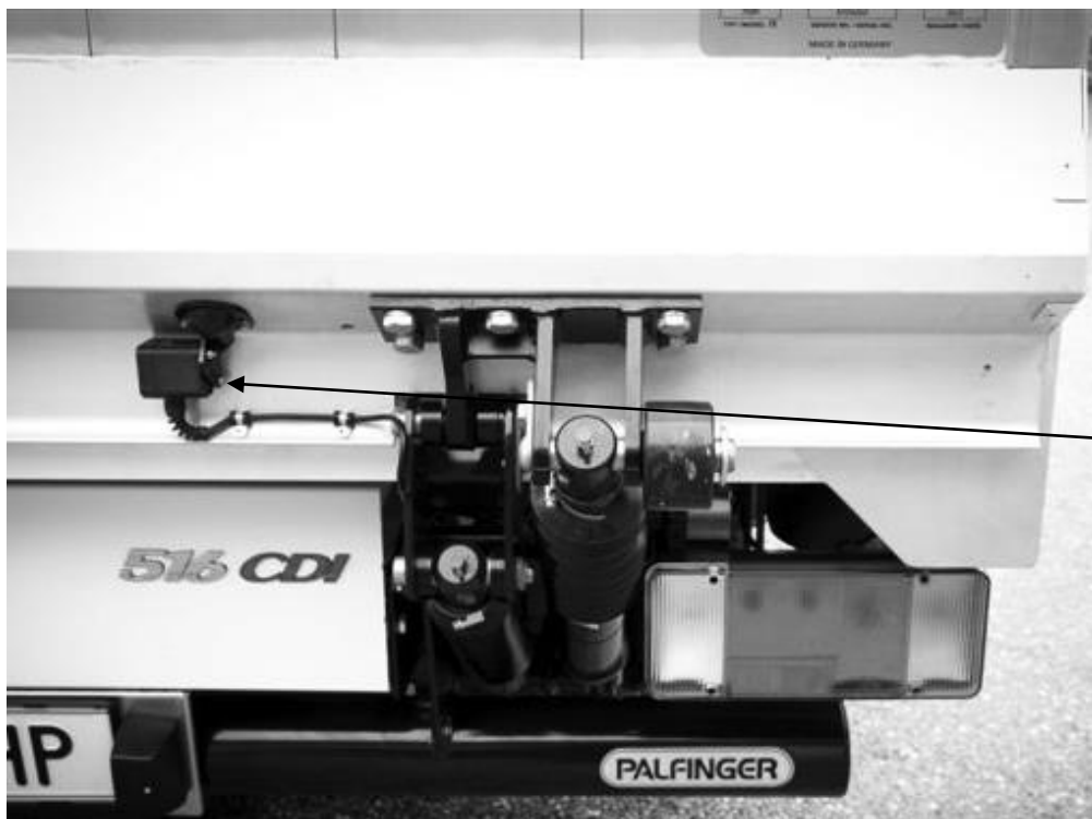
B-16 Sensor and warning light cable installation and placement
