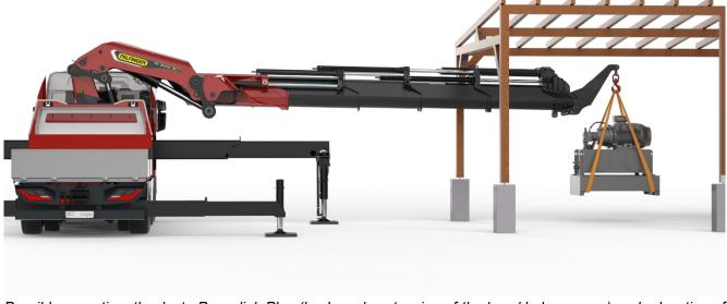
Possible operation, thanks to Powerlink Plus (backwards extension of the knuckle boom arm) and relocation of the anchor point. © PALFINGER
