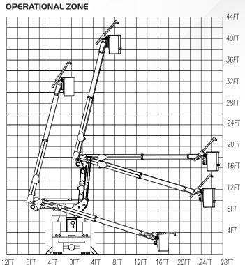
The ETC MH 37 IH insulated truck offers basket and turret full-pressure hydraulic controls with complete feathering capabilities and continuous rotation. The hydraulic winch and 5' jib allow up to 1,000 lbs. material handling, while the 24" x 30" bucket has tilt/rescue controls, engine start/stop, and a 90° rotator. Its two sets of outriggers, hydraulic tool circuit, jib extension, and 42' working height make PALFINGER's ETC MH 37 IH a powerful aerial unit.
