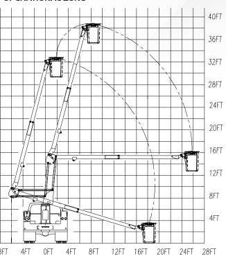
PALFINGER's non-insulated ETC 35 SNT offers standard 390° non-continuous rotation, emergency upper boom-controlled descent, adjustable wear pads, and replaceable bushings for pins. The 350 lbs. capacity bucket also features engine start/stop, hydraulic leveling, an extended gear-drive shaft for manual rotation, and variable speed controls.
