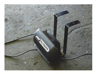
► Fix the control panel holder with screws or weld it in position as per the **PALFINGER Tail Lifts** assembly diagram.
