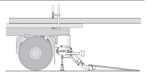
▶ Place two straight steel bearers of sufficient length on the load area between the control rod arms and vehicle body wall.
