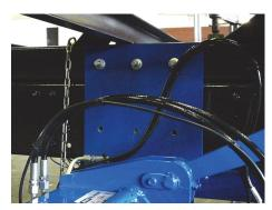
▶ Bolt the console plates to the vehicle chassis. In the process, note the tightening torques in the general assembly diagram and in the table on page 28.
