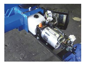
A slide-in unit is shown in the image. The oil level check is performed in a similar way for turning, box and universal units.
