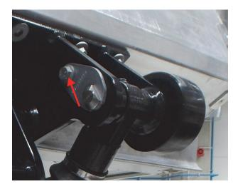
▶ Mount the floor roller and secure the pin with a snap ring.
