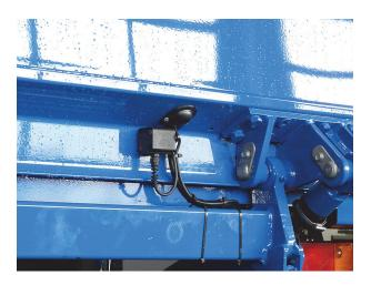
A tilt sensor b15 is shown in the image. The tilt sensor b16 is also mounted with the cable downwards.
