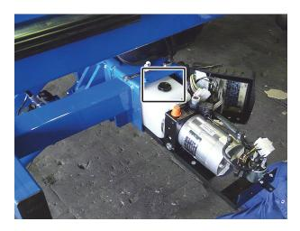
A slide-in unit is shown in the image. The air filter is inserted in a similar way for turning, box and universal units.
