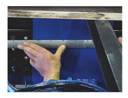
▶ Mark the following holes on the console plate. Observe the general assembly diagram and vehicle manufacturer's box body mounting guidelines. Above all, note the number, position and diameter of drill holes.
