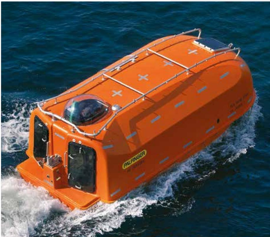
PALFINGER MARINE's totally enclosed lifeboats are designed and tested in accordance with latest IMO/SOLAS regulations. TECB Lifeboats are available in two versions: **Tanker and Dry Cargo.**
